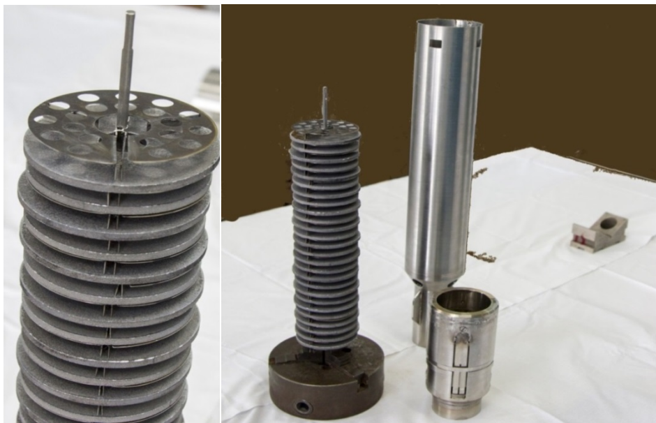
Figure 4. The irradiation device with chromium disks.
