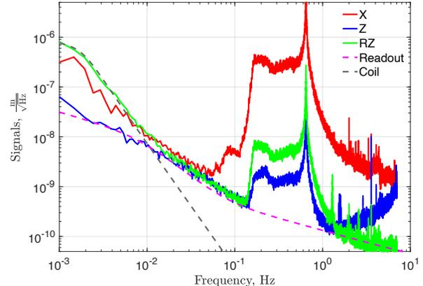
(b) Damped signals of the various degrees of freedom to highlight the noise floors due to sensing (Readout) and damping (Coil). Note that the Y and RX degrees of freedom are analogous to X and RY.
