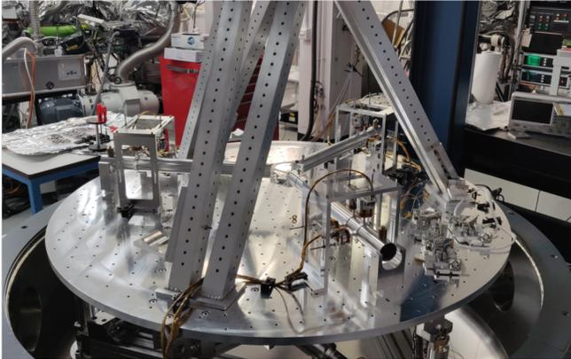
(a) Photo of experimental setup. The round active platform is stabilised relative to the seismometer with three arms.
