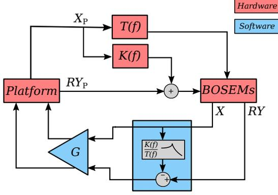
(a) Block diagram showing the feedforward scheme to subtract the translational induced tilt motion from the RY measurement.
