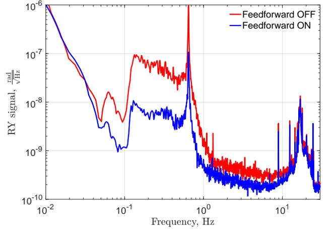
(b) Comparison of the RY signal with (blue) and without (red) feedforward of the X signal.
