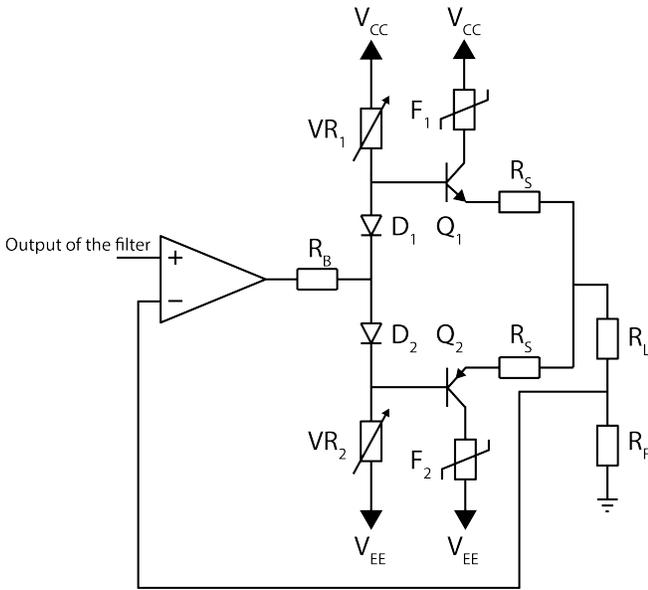
FIG. 2. Simplified schematic of a single output channel of the HCD. The design uses a class AB stage driven by an OPA2210 op-amp. Complete schematics and design files can be found on GitHub<sup>18</sup>
