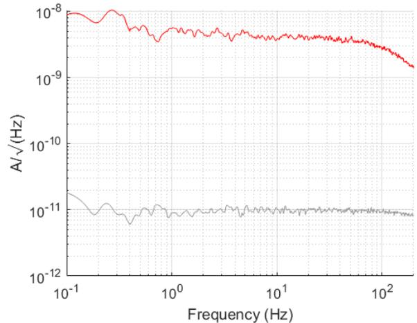
FIG. 5. NASD results in a bandwidth of 0.1 - 200 Hz for the HCD. 250 mA configuration (red) and noise floor of the setup terminated with 300  $\Omega$  resistor (light grey). Channel 3 is the only one shown to improve readability. Other channel results are presented in Table I. The NASD was obtained using logarithmic frequency axis power spectral density (LPSD) algorithm<sup>37</sup> made out of 2048 FFT points using Hann window with amplitude scaling correction applied.
