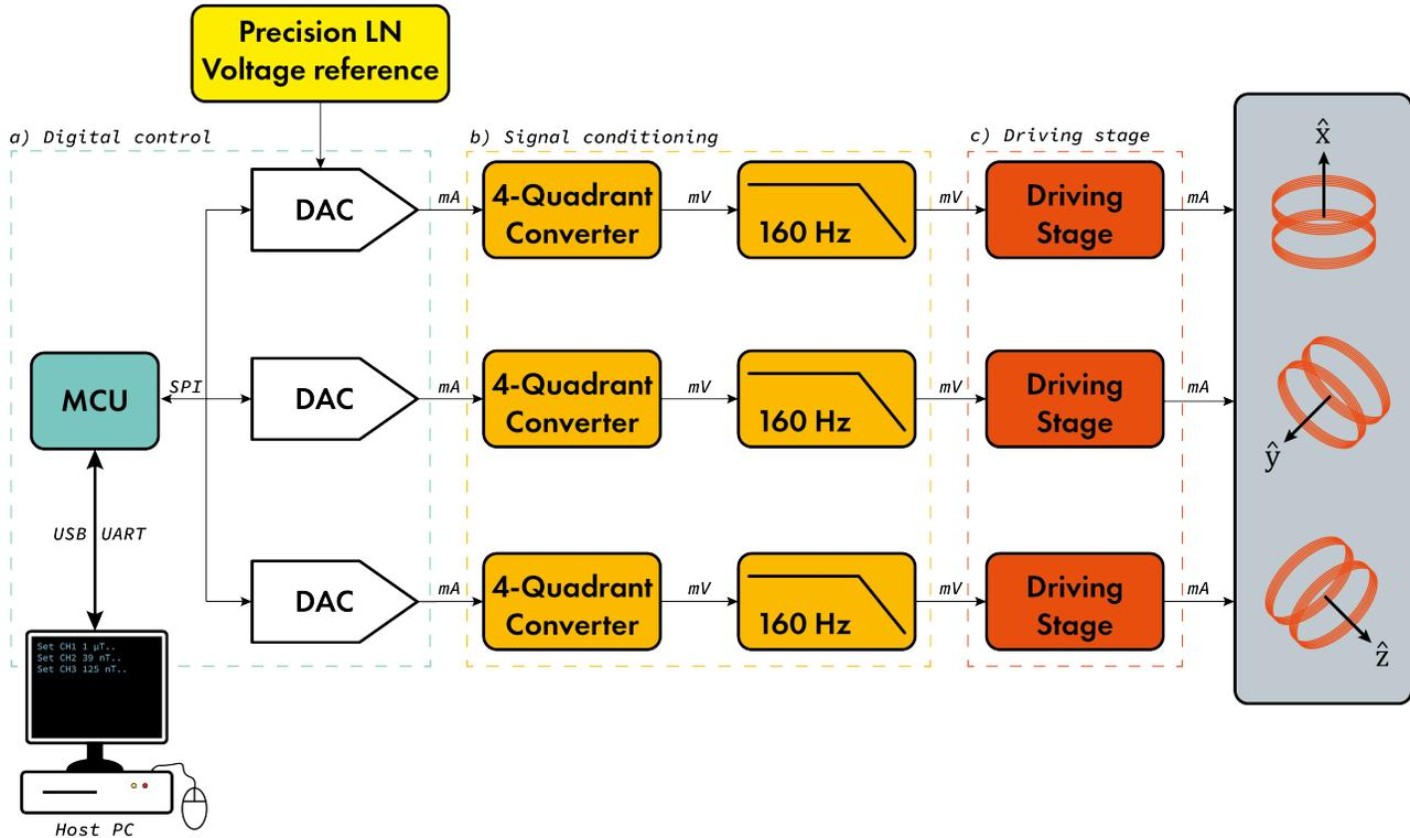
FIG. 1. Simplified architecture of the coil driver system. The design is split into three sections: (a) digital control, (b) signal conditioning, (c) and driving stage. The design is realised on a four-layer printed circuit board (PCB) with the signal conditioning and driving stages protected by EMI/RFI shielding. The design files, such as the schematic, board layout and bill of materials are available on GitHub<sup>18</sup>
