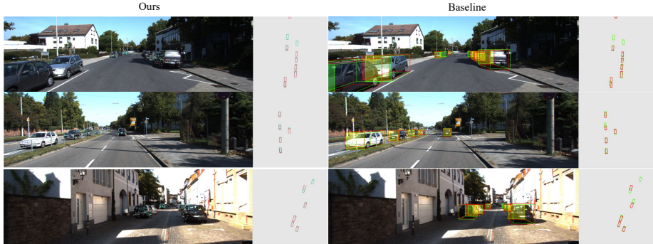
Fig. 3. The qualitative results on the KITTI val set. Rather than representing an object as a bounding box, we utilize semantic keypoints to represent an object. The red boxes represent the ground truth, while the green boxes represent the prediction.
