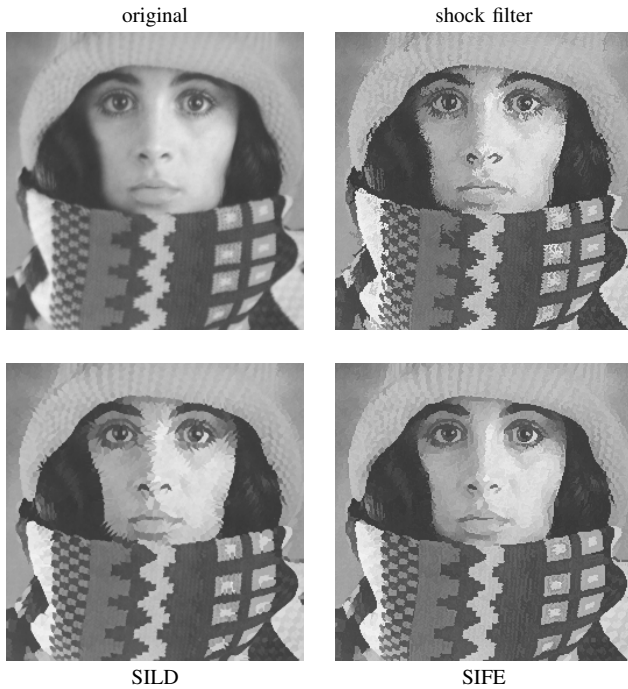
Fig. 1. Comparison of the steady states of shock filtering, SILD, and SIFE for the 256 \times 256 greyscale image trui .
