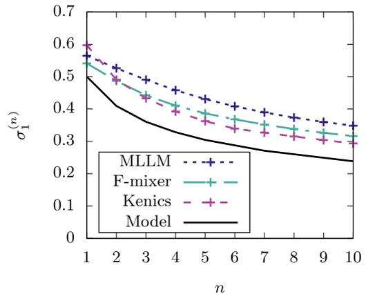
FIG. 7. Evolution of the mean absolute deviation  $\sigma_1^{(n)}$  with the number of elements  $n = 1, 2, 3, 4, 5, 7, 10$ , for the three mixers and the model.
