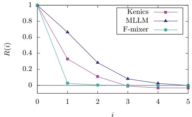
FIG. 2. Evolution of the correlation coefficient  $R(i)$  between residence time values in elements that are  $i$  elements away, for the three real mixers.
