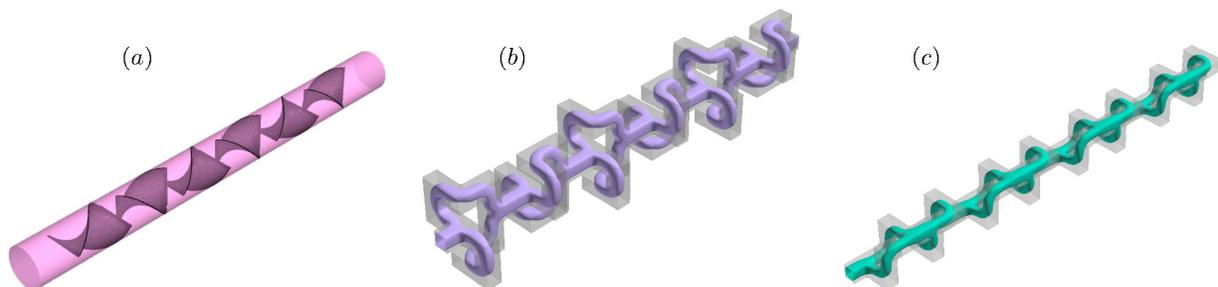
FIG. 1. Computational geometry of the different mixers studied: (a) the Kenics<sup>®</sup> mixer (6 elements); (b) the Multi-level laminating mixer (6 elements); (c) the "F" mixer (8 elements). For (b) and (c) an iso-surface of velocity modulus for a Stokes flow is plotted in color.
