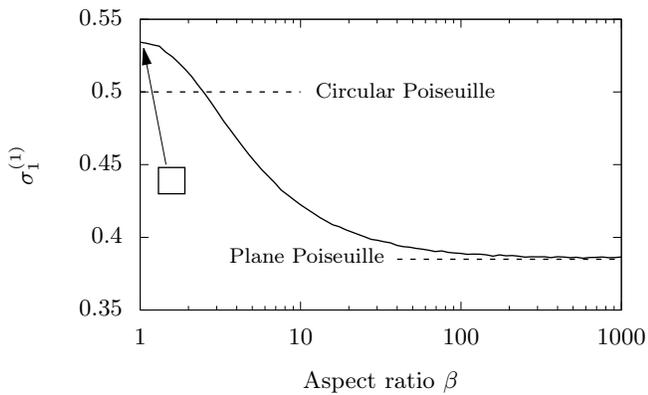
FIG. 8. Evolution of the mean absolute deviation for the Hagen-Poiseuille flow in rectangular ducts of varying aspect ratio  $\beta$ . Dashed lines indicate values of  $\sigma_1^{(1)}$  for the circular and plane Poiseuille flow configurations respectively  $\sigma_1^{(1)} = 1/2$  and  $\sigma_1^{(1)} = 2/(3\sqrt{3}) \simeq 0.385$ . As  $\beta$  increases, the configuration tends to that of the plane Poiseuille flow.
