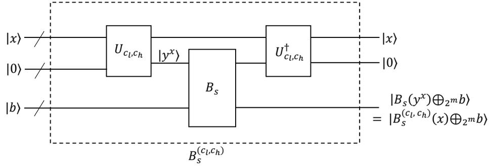
■ **Figure 2** The quantum circuit diagram implementing  $B_s^{(c_l, c_h)}$
