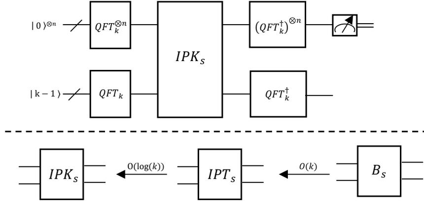
■ **Figure 4** The circuit diagram of Algorithm 7 is depicted above the dashed line. The idea of how to construct  $IPK_s$  is shown below the dashed line, where  $A \xleftarrow{O(t)} B$  means that  $A$  can be implemented by  $O(t)$  copies of  $B$ .
