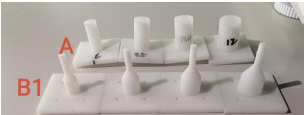
Figure S10. Device architecture and mesh holder. A schematic representing the assembly of the mesh in the holder (top) and different mesh holders used to evaluate the flow rate independence are shown (bottom).
