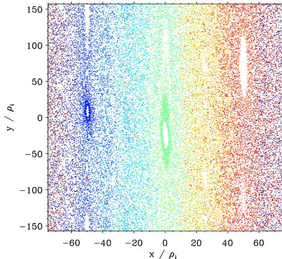
**Figure 1.** Poincaré plot of magnetic field lines intersecting the outboard midplane for the standard nonlinear simulation at  $tv_{th,i}/R = 1750$ .
