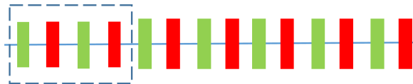
FIG. 4: Schematic plot of a FODO lattice used in the second application example. The four quadrupoles inside the dashed line box were used to match the initial distribution into the periodic FODO lattice.
