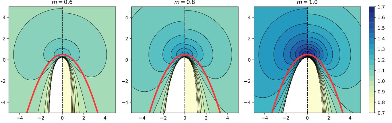
**Figure 5.** Density contours for three different values of the upstream Mach number  $m$ , in each case plotted using both the exact profile (Equation (79), left side) vs. the second-order polynomial approximation (Equation (82), right side). The red curves mark the parabolic obstacle. Density values below 0.7 are not shown, and no exact solution exists in the white region.
