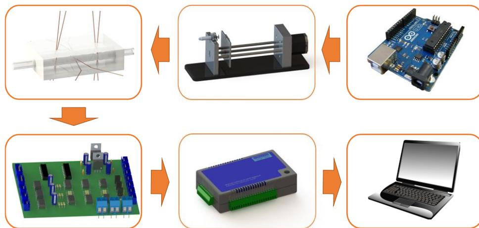
**Figure 5.** Experimental setup for evaluation of the fabricated chip
