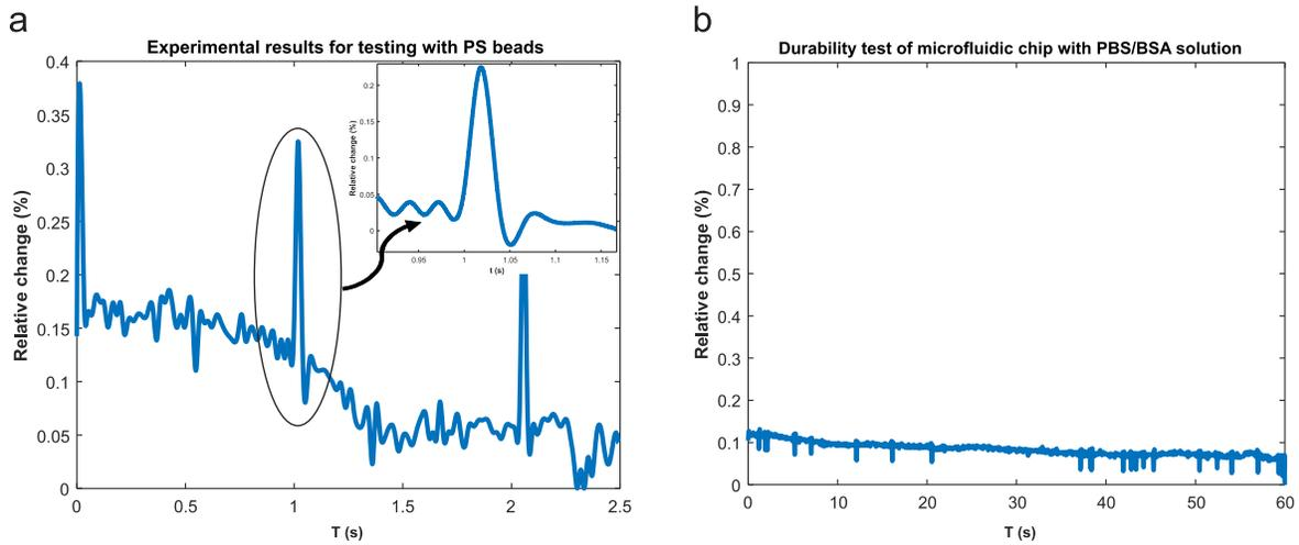
**Figure 8.** Experimental results of testing microfluidic chip with (a) PBS/BSA solution and 15 $\mu$ m PS beads. (b) PBS/BSA solution without PS beads
