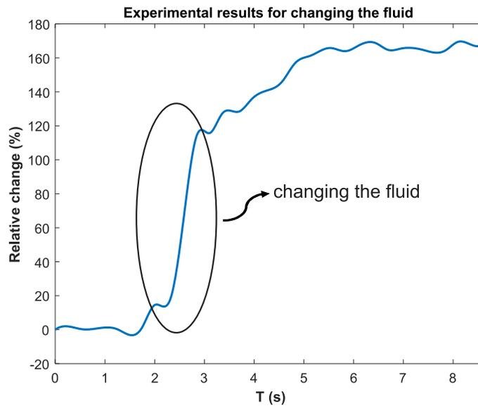
**Figure 7.** The experimental results of changing the fluid of the microfluidic channel from drinking water to PBS/BSA solution.
