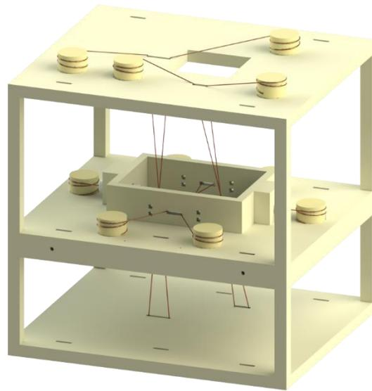
**Figure 1.** The 3D structure of the WWW method for rapid fabrication of microfluidic chips.
