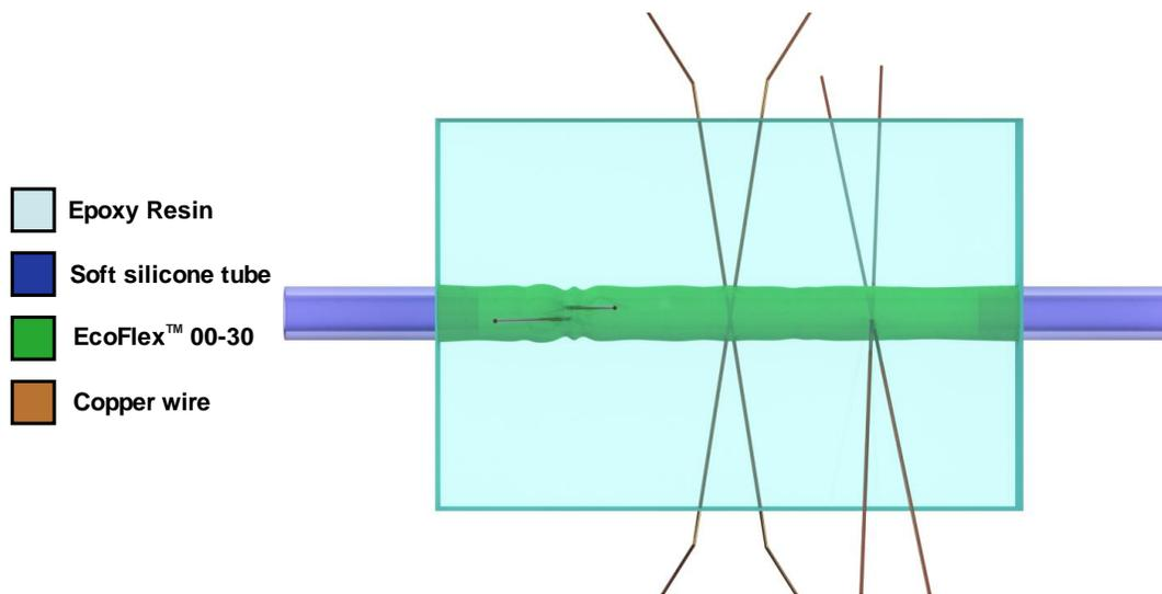
**Figure 3.** Schematic of the fabricated microfluidic chip with three pairs of 3D electrodes from the top view.
