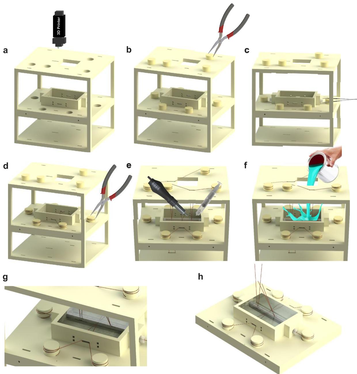
**Figure 2.** Fabrication procedure. (a) printing the structure using a 3D printer (b) fixing the cylinders (c) placing the soft silicone tube (d) wiring (e) making a rode of Ecoflex™ 00-30 using a syringe and curing the rod using a hot air gun (f) pouring the mold with Epoxy resin (g) putting the chip on the hot plate and wait to cure (h) detaching the 3D electrode wires from cylinders, disconnecting the inner and outer mold.
