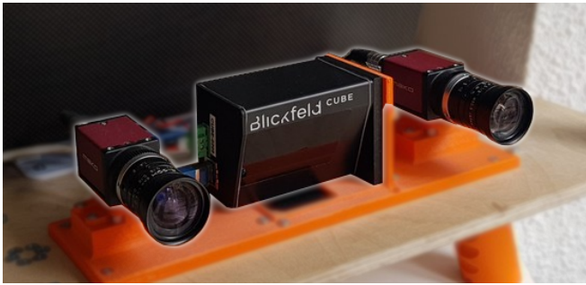
Fig. 3. The Stereo, Solid-State LiDAR, Inertial (S3LI) sensor setup
