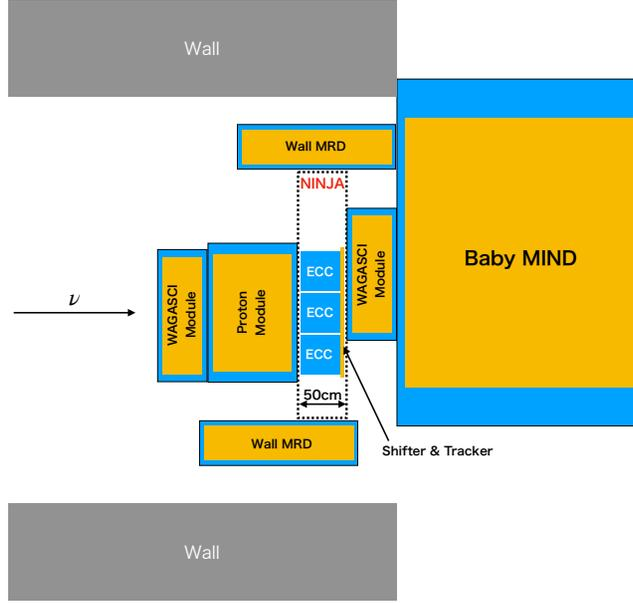
**Fig. 12** Detector setup of the NINJA experiment physics run viewed from the top. The NINJA detectors are surrounded by the WAGASCI detectors in the T2K experiment. The blue and orange regions show the total and scintillator volumes of each detector, respectively.
