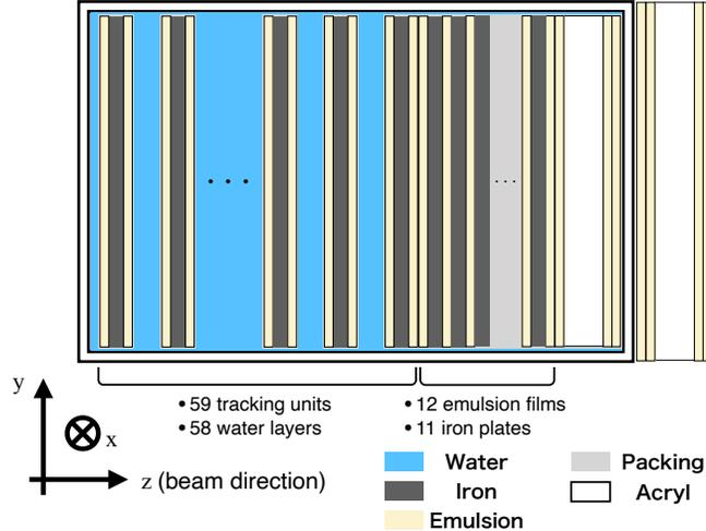
**Fig. 1** Water ECC used in the physics run of the NINJA experiment. Tracking units and 2.3 mm-thick water layers are alternately set perpendicularly to the neutrino beam direction. Each tracking unit consists of two emulsion films on both sides of a 500  $\mu\text{m}$ -thick iron plate.
