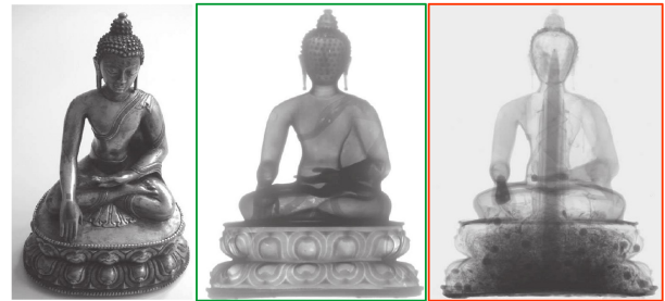
Figure 2: Optical (left), X-ray (middle) and neutron (right) imaging of a Buddha statue, from [2].
