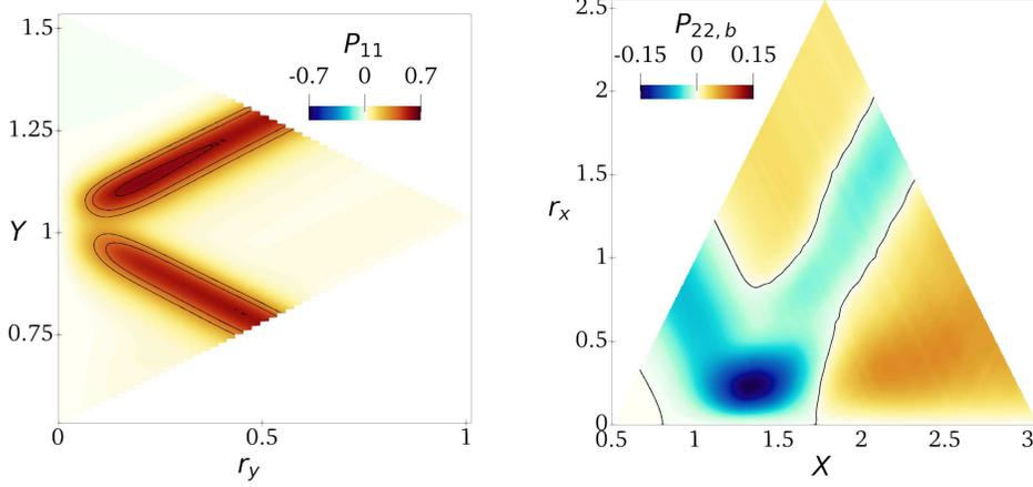
FIGURE 9. Production terms for  $\langle \delta u \delta u \rangle$  and  $\langle \delta v \delta v \rangle$  associated with the KH rolls. Left:  $P_{11}$  in the  $(Y, r_y)$  space with  $r_x = r_z = 0$ ,  $X = 1.5$  and  $0.5 \leq Y \leq 1.55$ . Right:  $P_{22}$  in the  $(X, r_x)$  space with  $r_y = r_z = 0$ ,  $Y = 0.99$  and  $0.5 \leq X \leq 3$ .
