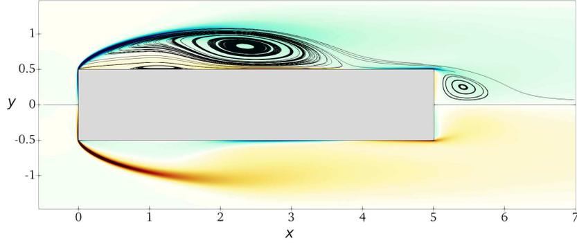
FIGURE 2. Mean streamlines (top half only) plotted over a colour contour of the mean spanwise vorticity  $\Omega_z$  (blue/red indicates negative/positive values in the range  $-20 \leq \Omega_z \leq 20$ ).
