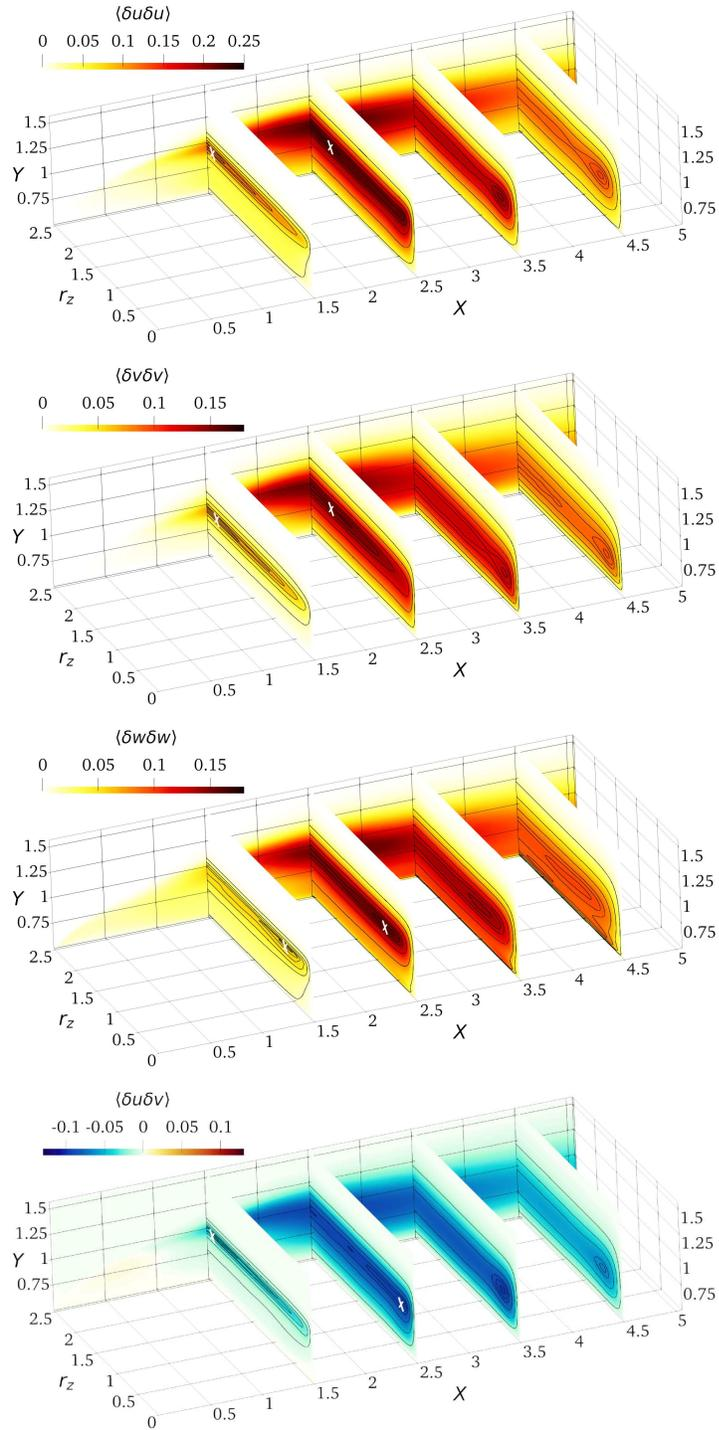
FIGURE 4. Components of the structure function tensor plotted in the space  $(X, Y, r_z)$  over the cylinder side. Contours in the planes  $X = 1.5, 2.5, 3.5, 4.5$  are for the 99%, 95%, 90%, 75%, 50% and 20% of the in-plane maximum. White crosses are used to identify local maxima when not easily visible.
