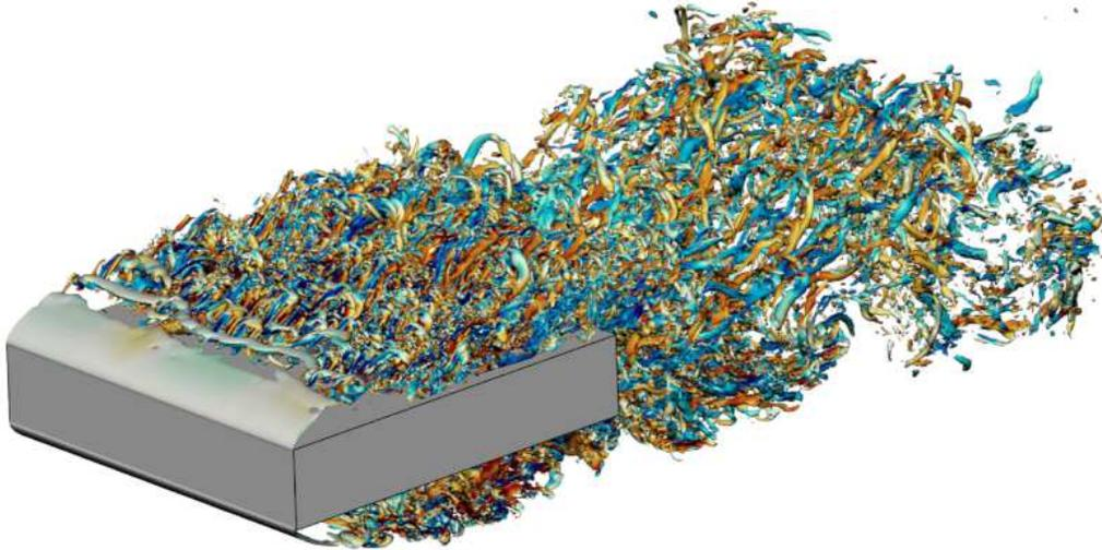
FIGURE 3. Instantaneous snapshot of the BARC flow: perspective view of the isosurfaces at  $\lambda_2 = -5$ . Color depicts streamwise vorticity  $\omega_x$ , with the blue-to-red colormap ranging in  $-10 \leq \omega_x \leq 10$ .
