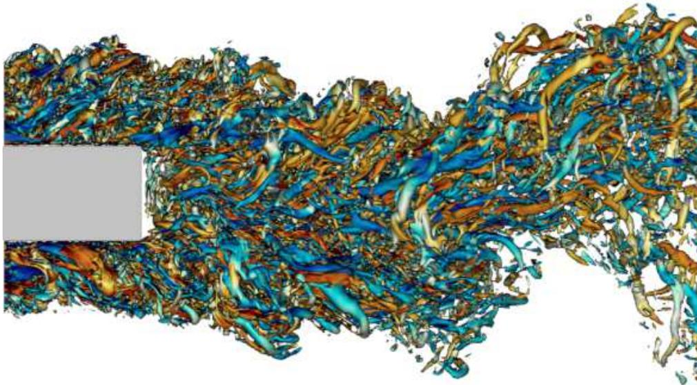
FIGURE 15. Instantaneous snapshot of the BARC flow: lateral view of the isosurfaces at  $\lambda_2 = -5$ , with zoom into the near-wake region. Colour depicts streamwise vorticity  $\omega_x$ , with the blue-to-red colormap ranging in  $-10 \leq \omega_x \leq 10$ . The vertical size  $D$  of the cylinder can be used as reference to identify the vertical and streamwise length scales of the near wake.
