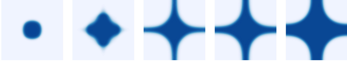
FIG. 20. Density contours in horizontal (y, z) planes for 3D RTI at At = 0.998 and Re = 3000 . t^* = 2 . k = 60, 120, 180, 240, 300 . The plane altitude is x = k/128 .
