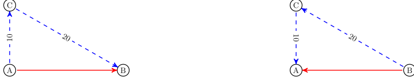
Figure 1: A couple of sorties, one being the inversion of the other. When w^{dr} = 10 , w_C = 5 and B = 350 , the sortie on the right is infeasible.
