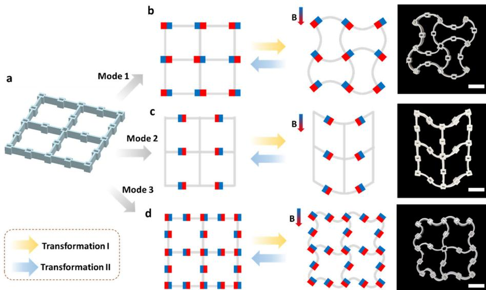
**Figure 3. Multimodal deformation of a square lattice with a different geometric arrangement of hard magnets:** (a) initial square lattice with pockets on the vertices and edges; (b) magnets on the vertices generate an achiral pattern – Mode 1; (c) magnets on the edge generate a bending pattern – Mode 2; (d) magnets on the vertices and edges generate a chiral pattern – Mode 3; the scale bar represents 10 mm.
