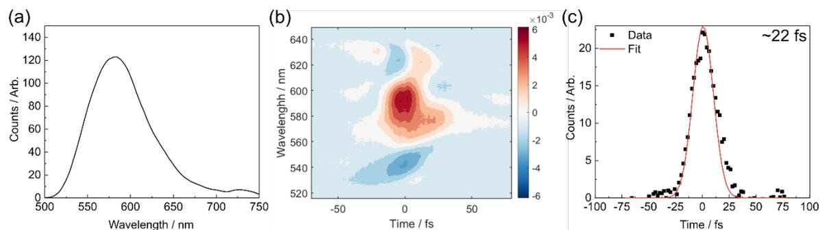
**Fig. S1** (a) Pump laser spectrum used in TA measurements, (b) Polarised-gating frequency resolved optical gating (PG-FROG) characterisation of pump pulses, (c) autocorrelation trace extracted from PG-FROG spectrum (square points) overlaid with Gaussian fit to data (red solid line).
