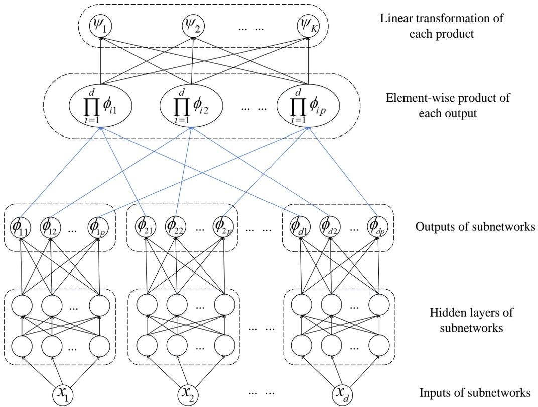
Figure 1: Architecture of  $K$ -dimensional output TNN. Black arrows mean linear transformation (or affine transformation). Each ending node of blue arrows is obtained by taking the scalar multiplication of all starting nodes of blue arrows that end in this ending node.
