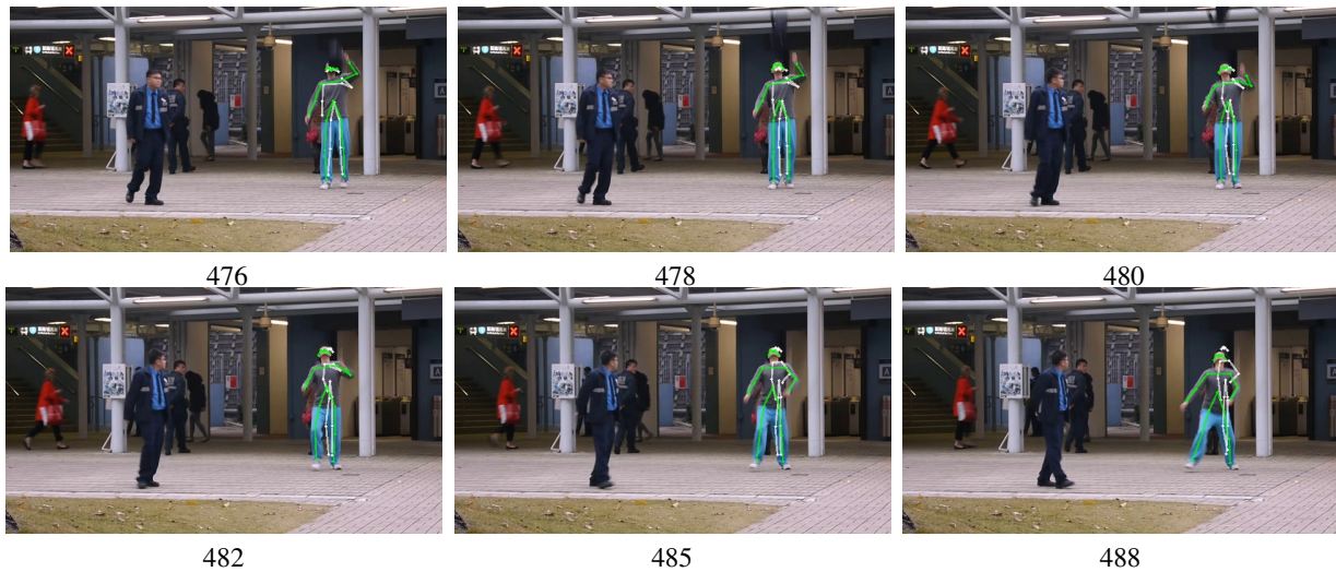
Figure 4. Visualization of ground truth (green) and predicted poses (white) for an anomalous activity, where the pedestrian is jumping up and also throwing a bag (timescale 13, Avenue dataset video 05 frames #467 to #488, pedestrian ID 06). Best viewed in color. The numbers under the images are frame numbers.
