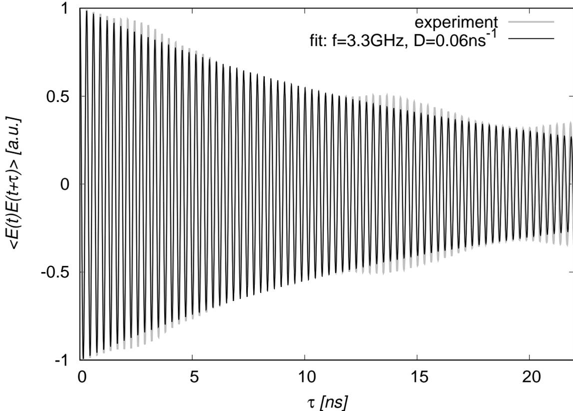
Figure 3: Normalized autocorrelation function.
