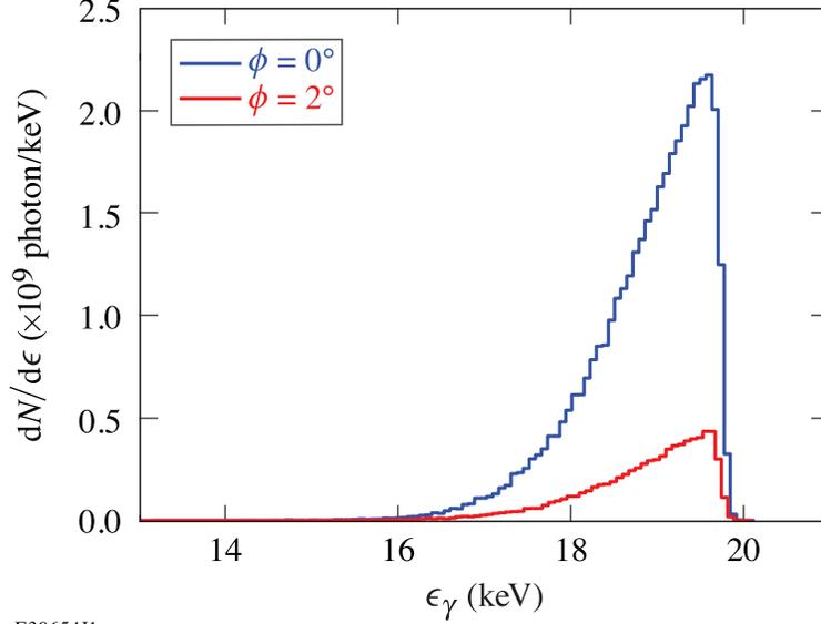
FIG. 3. X-ray photon spectra of the Gaussian laser configuration, with crossing angles of  $0^\circ$  and  $2^\circ$ . The number density of scattered photons is plotted against the scattered photon energy.
