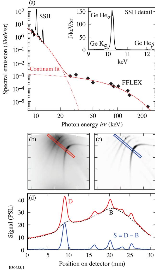
FIG. 6. X-ray diffraction data collected on the NIF. (a) The 11-keV x-ray line of interest (Ge  $He_\alpha$ ) sits on a two-exponential background containing a similar amount of energy ( $E_{BG}/E_{line} \approx 80\%$ ). (b) The raw data require (c) background subtraction to obtain (d) analyzable diffraction lines. The signal-to-background ratio is often below unity, obscuring small peaks and detail in the signal. Images reproduced with permission from Ref. [44].
