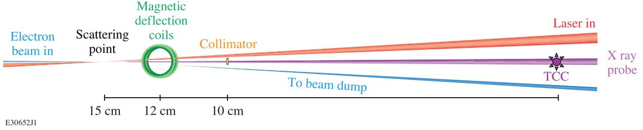
FIG. 4. Cartoon of laser-electron interaction region for case with the final laser optic on the opposite side of TCC from the electron beam. This image assumes  $\phi = 2^\circ$  and electron deflection angle  $3^\circ$  ( $B \sim 1$  T).
