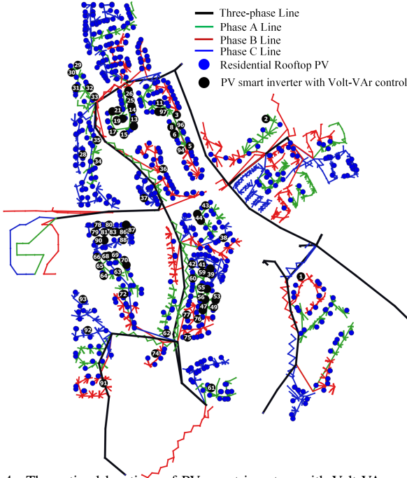
Fig. 4. The optimal locations of PV smart inverters with Volt-VAR control
