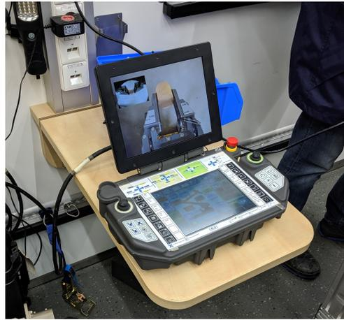
Fig. 2: The Telemax OCU with a touch panel in the middle and a monitor for video feedback. It can also be connected to an external screen.
