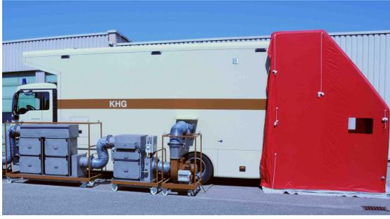
Fig. 3: The truck that houses the mobile control room, including the mobile air filtering system and the red inflatable tent used as an entrance.
