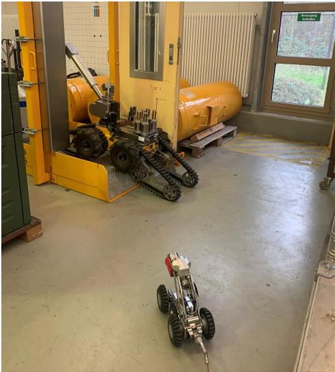
Fig. 5: Telex and the reconnaissance robot during the second mission. The second robot provides an additional viewpoint for the operator.
