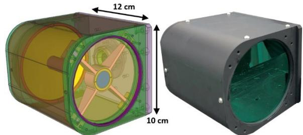
Fig. 3. 3D model and prototype of the 9-cm telescope.
