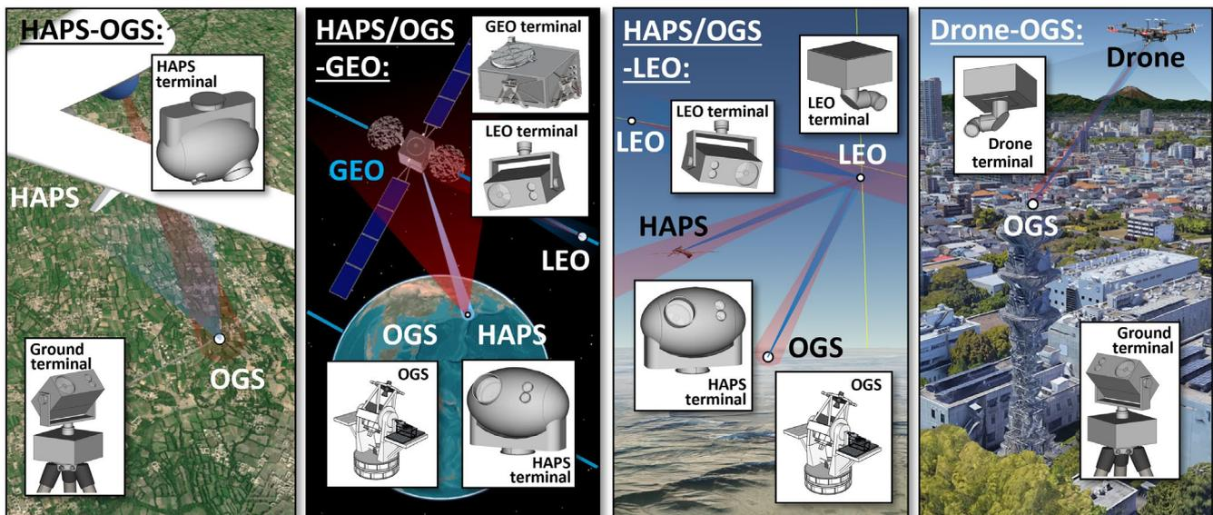
Fig. 1. Use-case examples of NICT's lasercom terminals in a variety of different scenarios and platforms.
