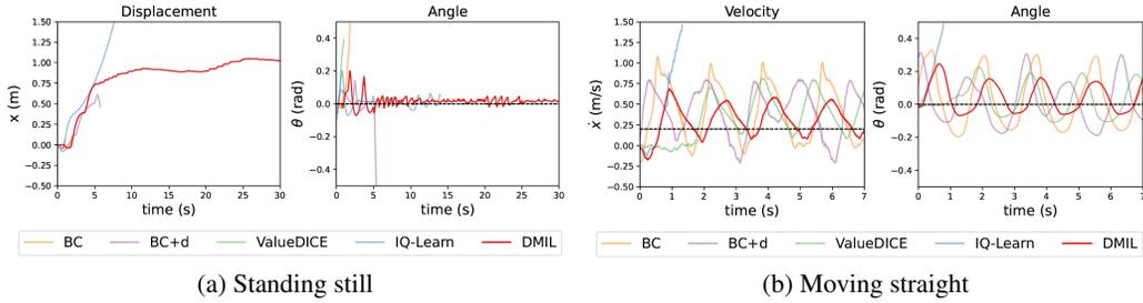
Figure 4: Evaluation results on a real-world wheel-legged robot
