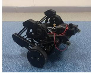
Figure 3: Wheel-legged robot
