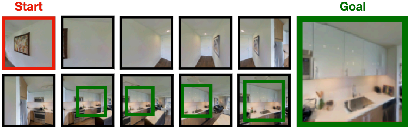
Fig. 1: A rollout of our navigation policy pre-trained with random crop prediction on synthetic noise images . Given a goal image and the current view, the agent first explores the environment by panning its camera. Once the goal view is detected, shown by the green bounding box, the agent moves towards the goal to complete the task. Click the image for a video.
