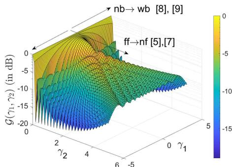
Fig. 1. 3D plot of  $\mathcal{G}(\gamma_1, \gamma_2)$  vs  $\gamma_1$  and  $\gamma_2$  in dB scale. Increase in  $|\gamma_1|$  corresponds to transition from narrowband to wideband; increase in  $\gamma_2$  corresponds to transition from far-field to near-field.
