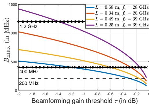
Fig. 4.  $B_{\max}$  as a function of the beamforming gain threshold for  $\{L, f_c\} \equiv (0.68 \text{ m}, 28 \text{ GHz}), (0.34 \text{ m}, 28 \text{ GHz}), (0.49 \text{ m}, 39 \text{ GHz}), (0.25 \text{ m}, 39 \text{ GHz})$ . Tradeoff between gain threshold and maximum usable bandwidth is illustrated.
