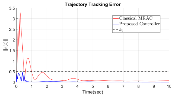
Fig. 1. Comparative analysis of trajectory tracking error using the proposed control law (21) and classical MRAC law (8).
