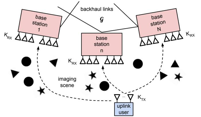
Fig. 1. System configuration with  $N$  base stations receiving transmissions from an uplink user. Base stations are connected over static, undirected backhaul network  $\mathcal{G}$ . Base stations aim to collaboratively image the scene and perform uplink user symbol detection.
