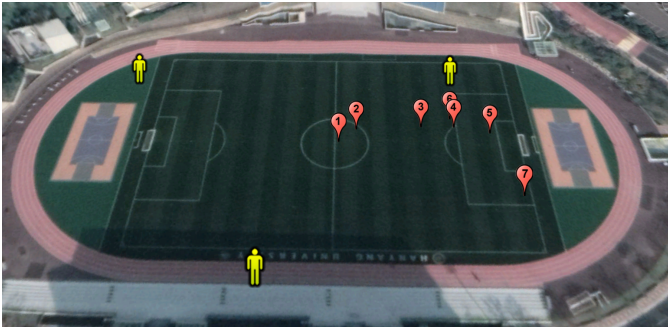
Fig. 1. An open space test environment. The yellow icons represent the receivers and the red icons represent the positions of the target.
