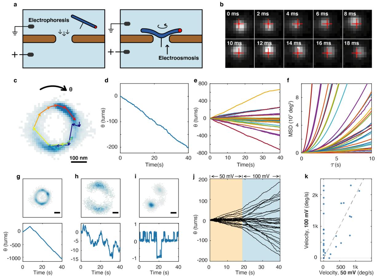
**Fig. 2. Unidirectional rotation of a DNA rotor under a transmembrane voltage.**
