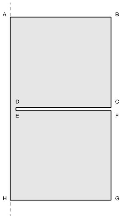
**Fig. S12. Geometry used in simulating electroosmotic flow through the nanopore.** ABHG denotes an XZ plane across the nanopore axis AH for a nanopore that is located midway between A and H. Rotation symmetry defines the electroosmotic flow in 3D by rotating this plane about the AH axis.
