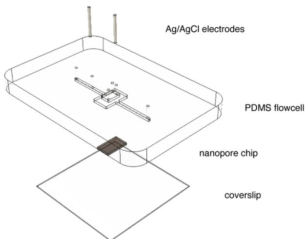
**Fig. S14. Schematic of the PDMS flow cell used in the experiments.**
