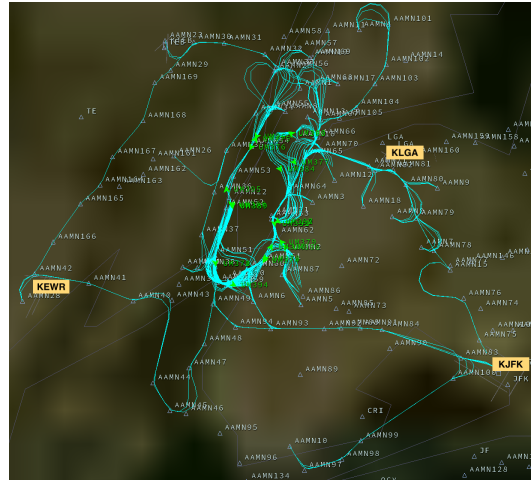
Fig. 2. Simulated AAM traffic in the NYC area displayed in the BlueSky air traffic simulator. Blue lines represent flown AAM trajectories. Green arrows represent AAM traffic currently in-flight.
