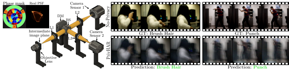
Fig. 6. Experimental setup scheme and some results on acquired videos. The deformable mirror configuration and characterized PSF are shown in the upper left corner. The right column shows the non-privacy and private videos obtained with our camera.
