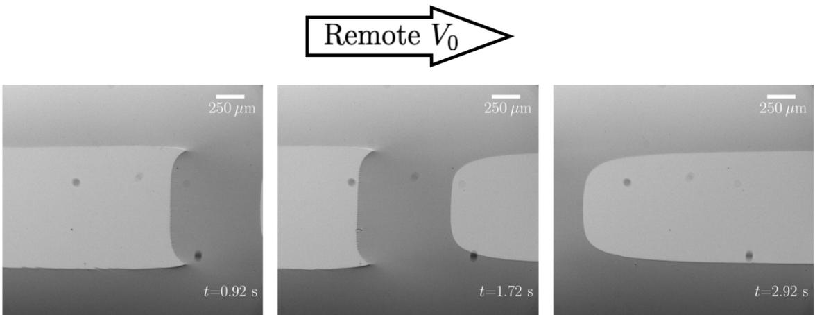
Figure 6: Propagation of the dual of the Schallamach wave or the separation pulse. Remote sliding  $V_0$  occurs in the same direction as before, but the detachment wave moves in the opposite direction. Despite this, slip occurs in the same direction as the applied  $V_0$ . Note that, just as with the Schallamach wave, this separation pulse also propagates at speeds much lesser than elastic wave speeds.
