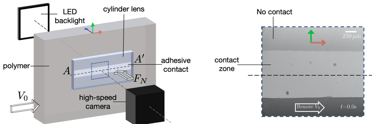
Figure 4: Experimental schematic showing a typical cylindrical lens in adhesive contact leading to the formation of an ‘adhesive’ channel. The schematic on the left shows a typical configuration with a backlit source and remote applied motion  $V_0$ . A sample image showing the contact zone (light grey) and detached zones (dark grey) is presented in the right panel. Note that the red, green and blue arrows represent the  $x$ ,  $y$ ,  $z$  axes, respectively.
