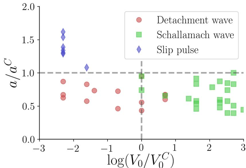
Figure 9: A two-parameter phase diagram showing domains of occurrence of the three Schallamach-type waves discussed in the article. Schallamach waves occur above a critical sliding velocity, separation pulses occur at a low  $V_0$  and normal loads while detachment-less slip pulses mediate motion at large normal loads.
