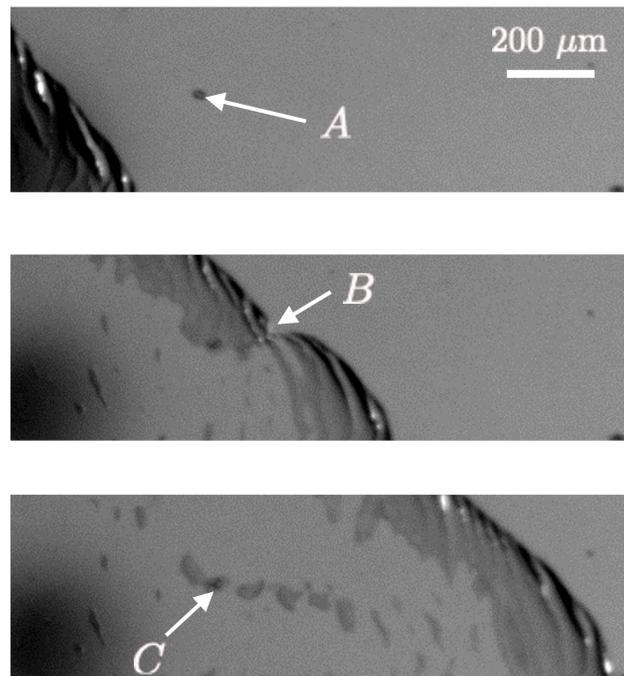
Figure 11: Interaction between a solitary Schallamach wave and a large dirt particle  $A$  on the interface. The wave approaches the particle and is bowed by it (at  $B$ ), following which a residual detachment region is left behind ( $C$ ) around the dirt particle. This outcome is also analogous to that observed during dislocation-point defect interaction.
