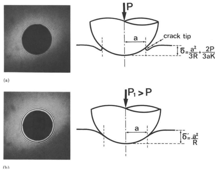
Figure 2: Schematic comparing standard Hertzian non-adhesive contact (bottom) and JKR-type adhesive contact (top). In the former, the rubber surface is nearly tangential to the indenter profile. In the latter, it is normal to the surface, due to intermolecular attraction. Adapted from Ref. [17].
