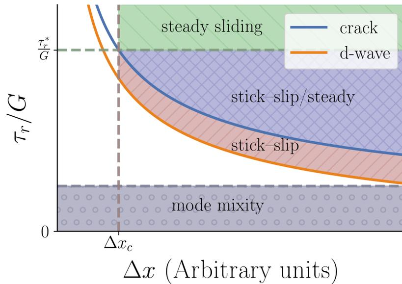
Figure 12: Qualitative phase diagram comparing Schallamach-type detachment waves with shear cracks to predict when stick-slip should occur at the expense of steady sliding. The orange curve (d-wave) represents the equivalent stress intensity factor for a moving detachment wave ( $\nu = 0.5$ ) while the blue curve is for an equivalent shear crack of the same initial extent. The shaded regions are labeled based on which phenomenon, stick-slip or steady sliding/crack growth, is expected to occur.
