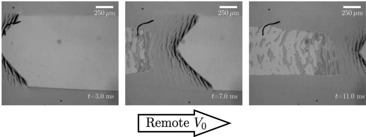
Figure 5: Evolution of a single Schallamach wave under remote applied  $V_0$  to the elastic polymer. The wave propagates from left to right, in the same direction as  $V_0$  and causes slip in its wake. The interface is stationary before and after the wave has passed. This is seen by following the motion of a dirt particle (black line) embedded on the polymer sub-surface. The scale bar and timestamp shows that the wavespeed is much lesser than typical elastic wave speeds.
