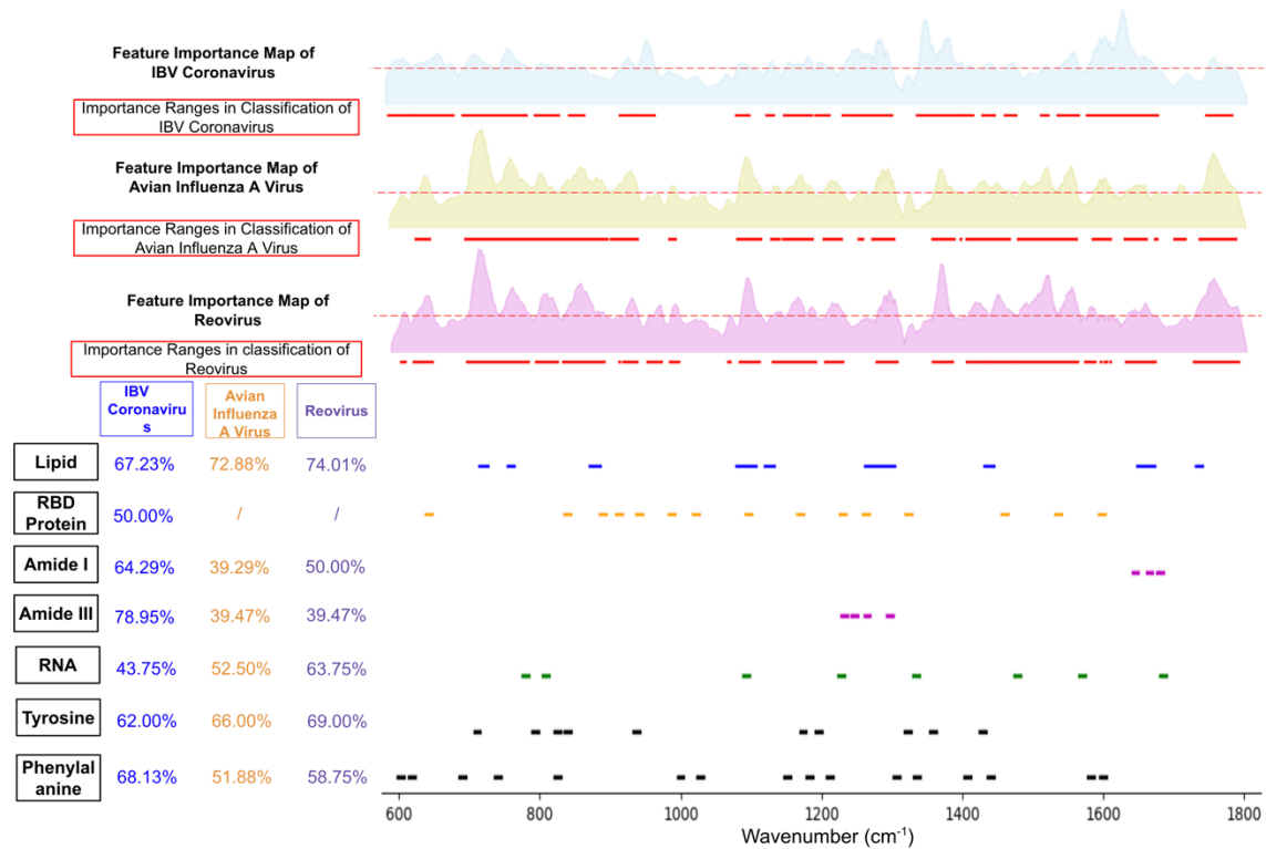
Figure 8. ML-calculated feature importance map, and important Raman ranges for classifying three types of avian viruses: IBV Coronavirus, Avian Influenza A virus and Reovirus. Feature important maps and matching scores are given for each avian virus type. The matching score for RBD Protein only applies when correlating with IBV Coronavirus because RBD Protein is an exclusive biomolecule in IBV. (See SI Appendix , Fig. S2 for matching scores with more functional groups).
