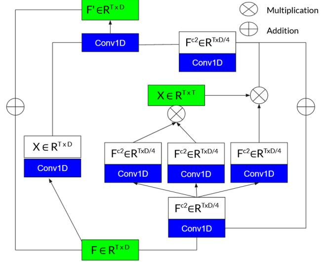
Fig. 2. The proposed attention layer architecture
