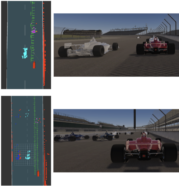
Fig. 5. LiDAR Point Classification Examples: Visualization Plots (left), Corresponding Simulation Screenshots (right). Points with different colors belong to different lanes.
