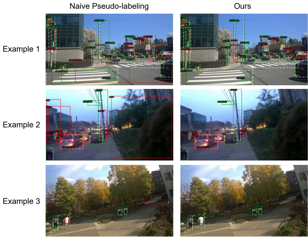
Figure S2. Visualization of example pseudo-labels predicted by our Efficient-CLS and the Naive Pseudo-labeling. The white box with dash line denotes the ground truth label. The box with solid line denotes the pseudo-labels (the ones in green are correct while the red are wrong labels). The Naive Pseudo-labeling only has one learner and uses the pseudo-labels generated by itself for training.
