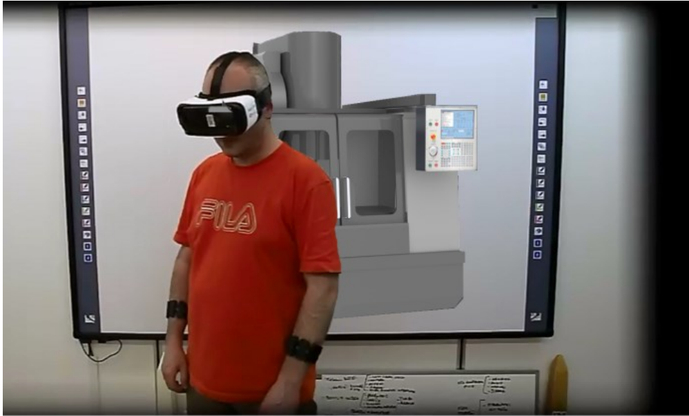
Figure 12: SOPHOS-MS integrated with immersive headset, interactive whiteboard and motion capture armbands
