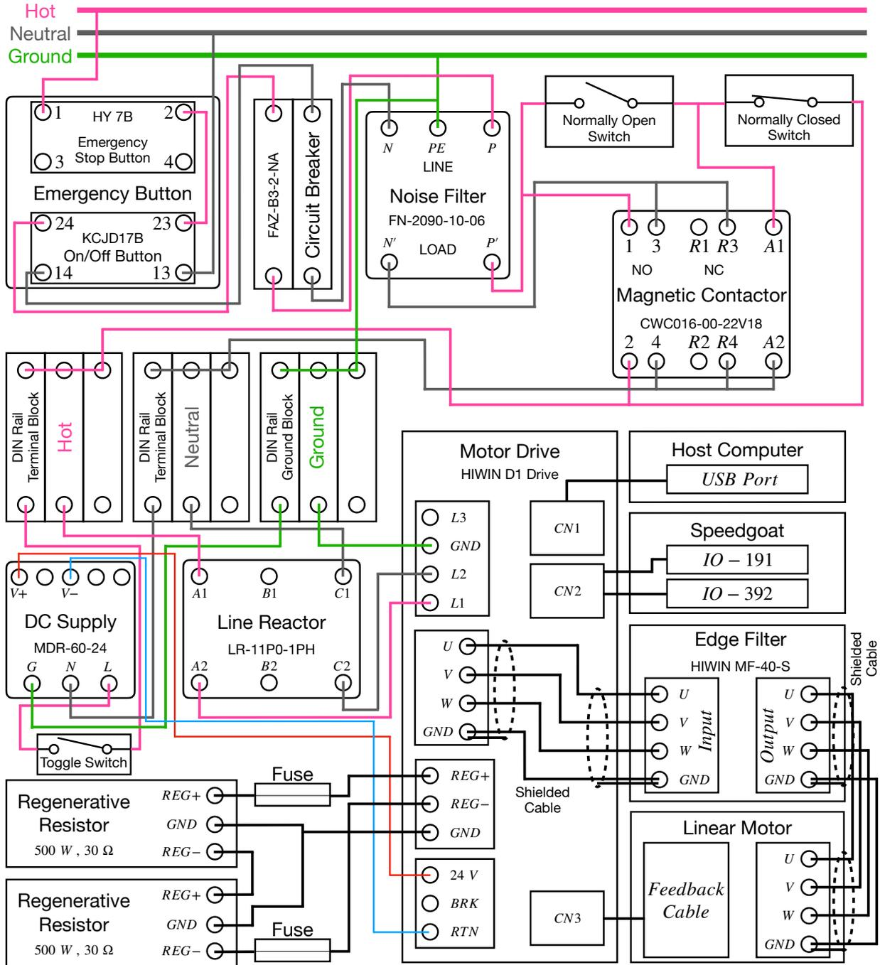
Figure 24: This figure illustrates the overall electrical components needed to provide power supply to the linear motor. An electrical box is used to put all the components together.
