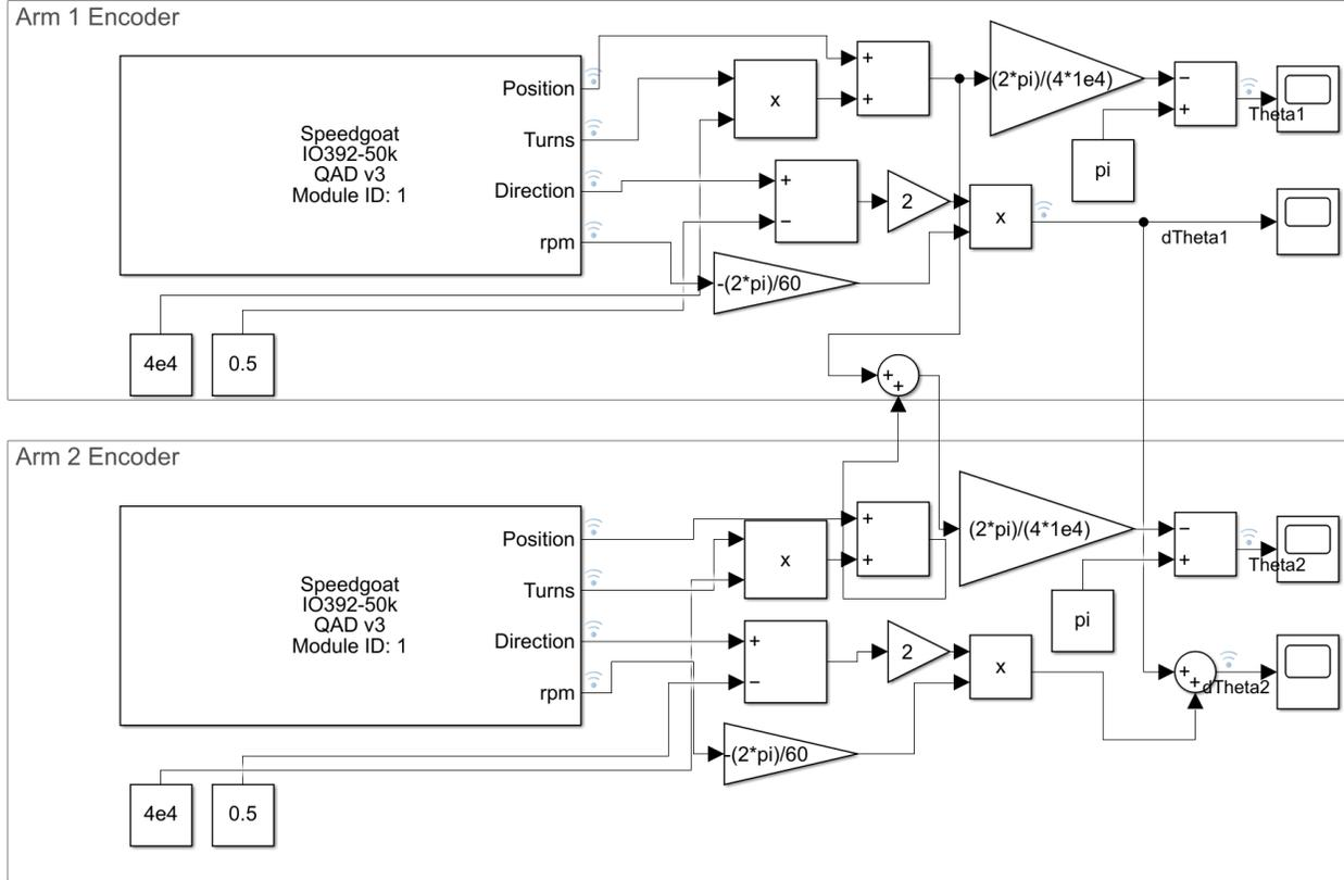
Figure 38: This figure illustrates how to read the angular position of the double pendulum shown in Fig. 1. Conversion in Eq. (5) and Eq. (6) is needed to read the angular position of the second pendulum arm defined in Fig. 1. A similar configuration of the encoder block is performed as we did in Fig. 37 with a different value for the "Steps per revolution vector" blank.
