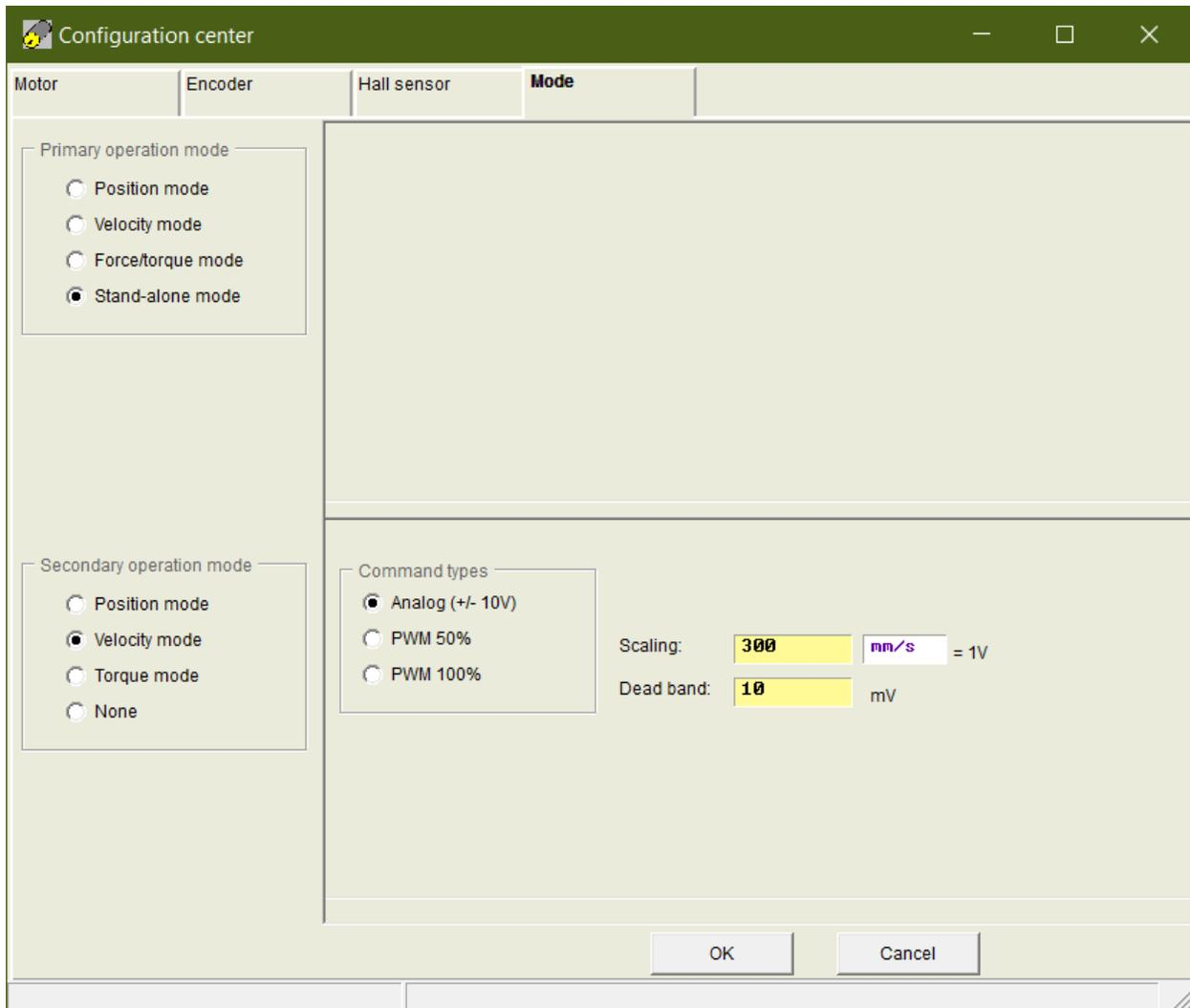
Figure 29: This figure illustrates the selection of the linear motor’s operating mode.
