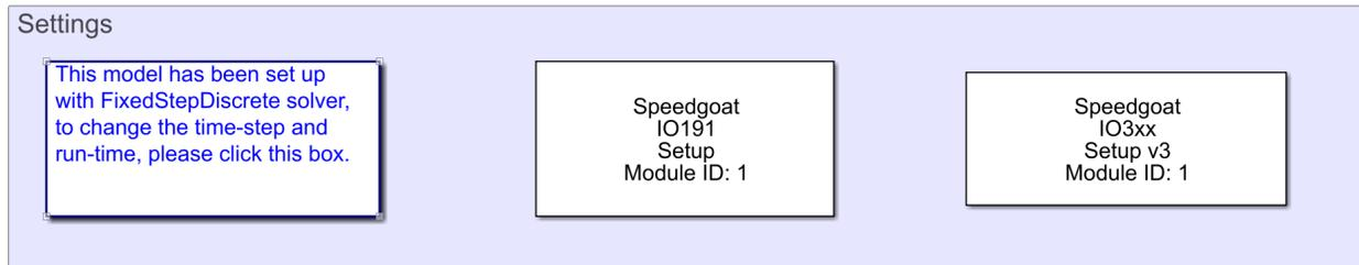
Figure 33: This figure illustrates the two block sets used in the Simulink model that configures the Speedgoat IO-191 and Speedgoat IO-392 modules.
