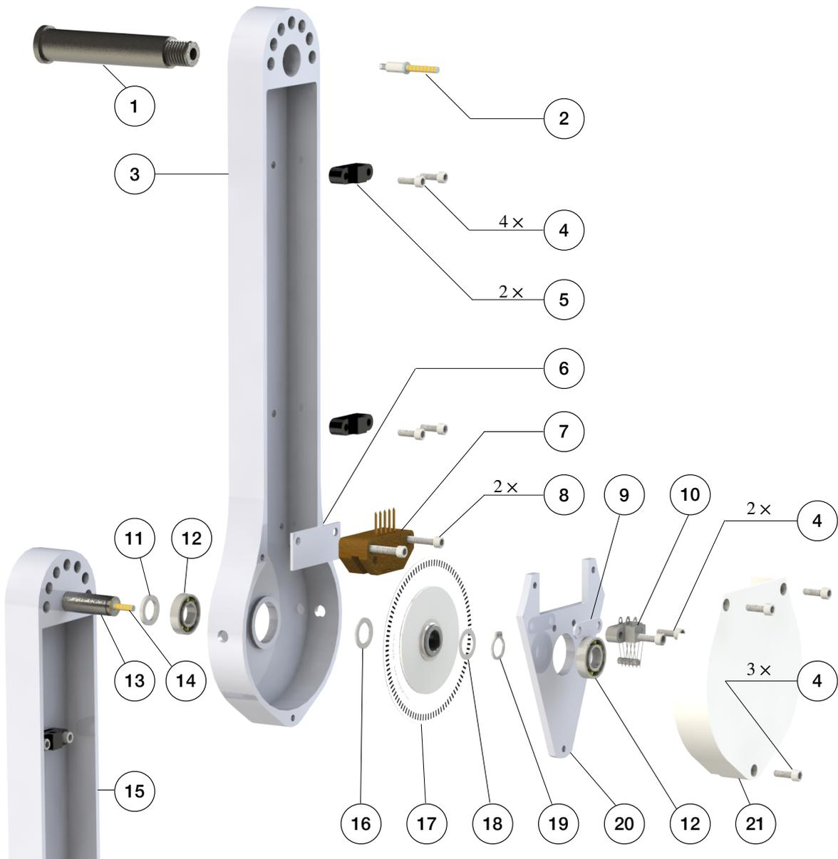
Figure 5: Components and assembly of the first and second pendulum arm.
