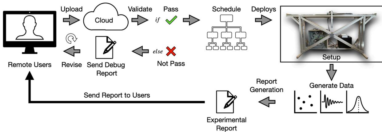
Figure 13: Overall schematic of a cloud experiment of the pendulum on the cart system.
