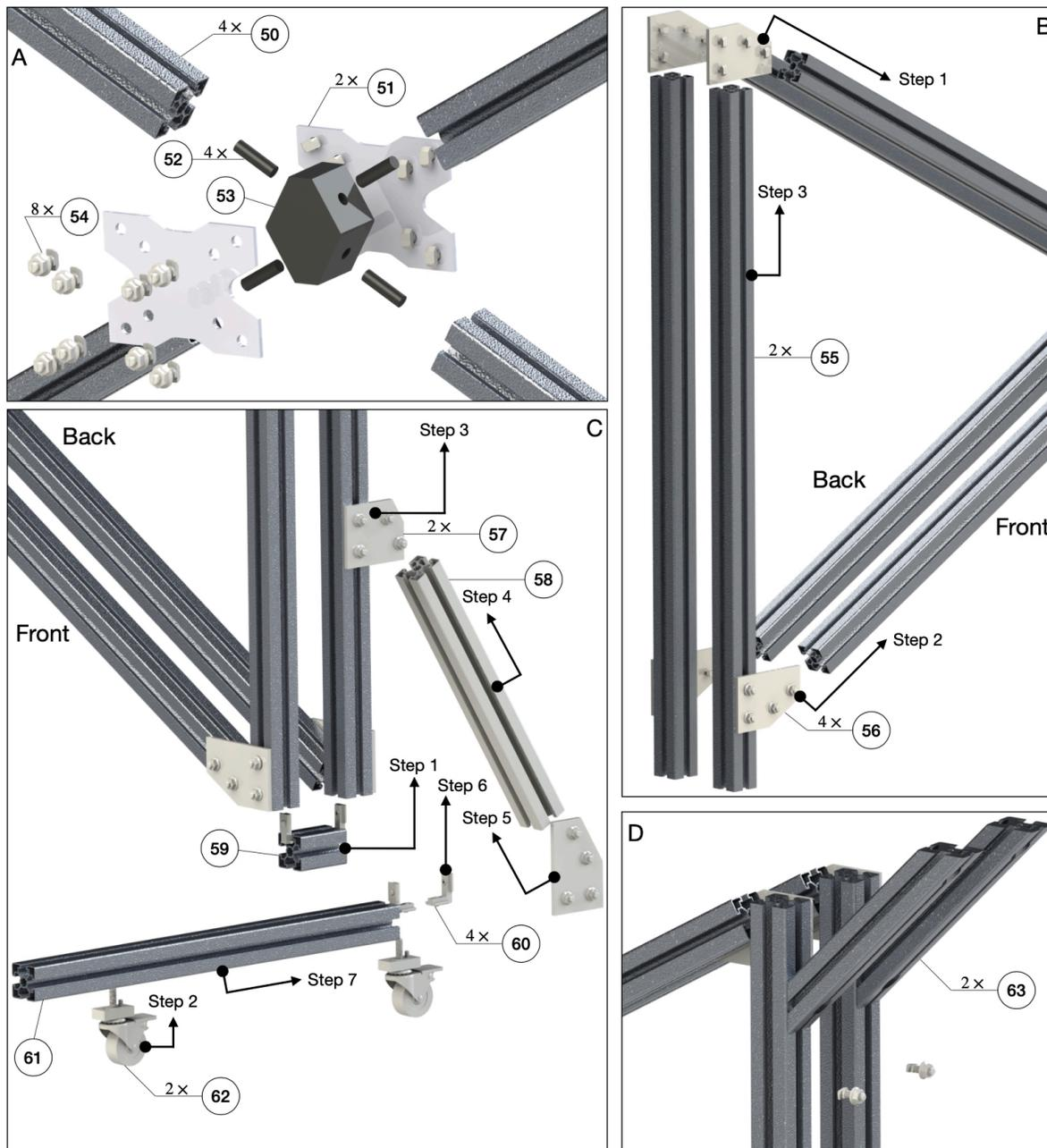
Figure 21: Assembly of the system frame. (A) Installation procedure of the X shaped frame. (B) Connection of the X shaped frame with the vertical aluminum extrusion (55). (C) Installation of the wheel to the system frame. (D) Installation of diagonal brace.
