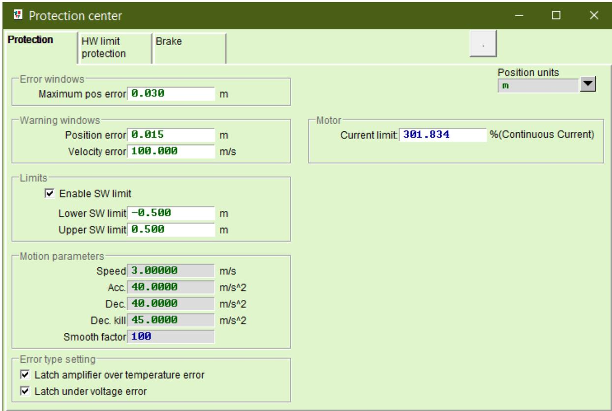
Figure 32: This figure illustrates the software safety configuration by using Lightning software.
