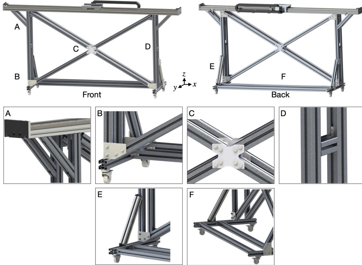
Figure 20: System frame. The linear motor is lifted up using four vertical aluminum extrusion. Different aluminum extrusions are installed to constrain the movement of system frame in the  $x - z$  and  $y - z$  plane. To allow easy moving of the experimental setup, four wheels can be installed to the system frame as shown in (E) and (F).
