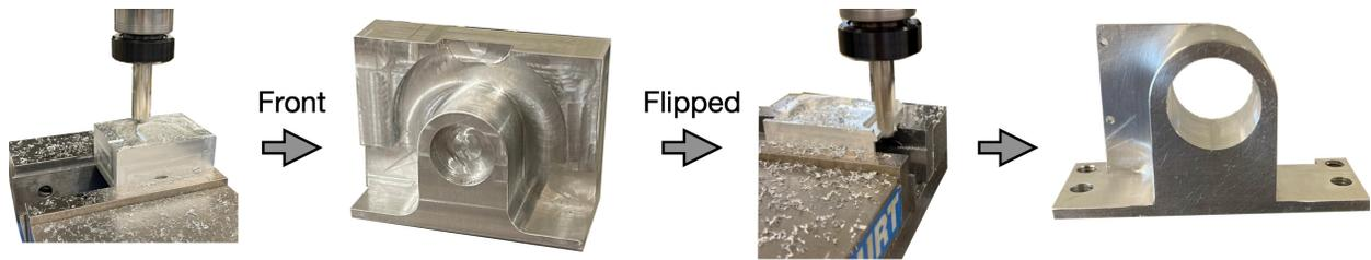
Figure 19: This figure illustrates the overall process of machining the bearing housing. To start with, the aluminum cube is face milled to create the datum face. Then the features on the front of the bearing housing is machined. Next, the aluminum cube is flipped over to machine the features on the backside of the aluminum cube and all the necessary holes needed are drill. Finally, the bearing housing is polished and sharp edges are smoothed.
