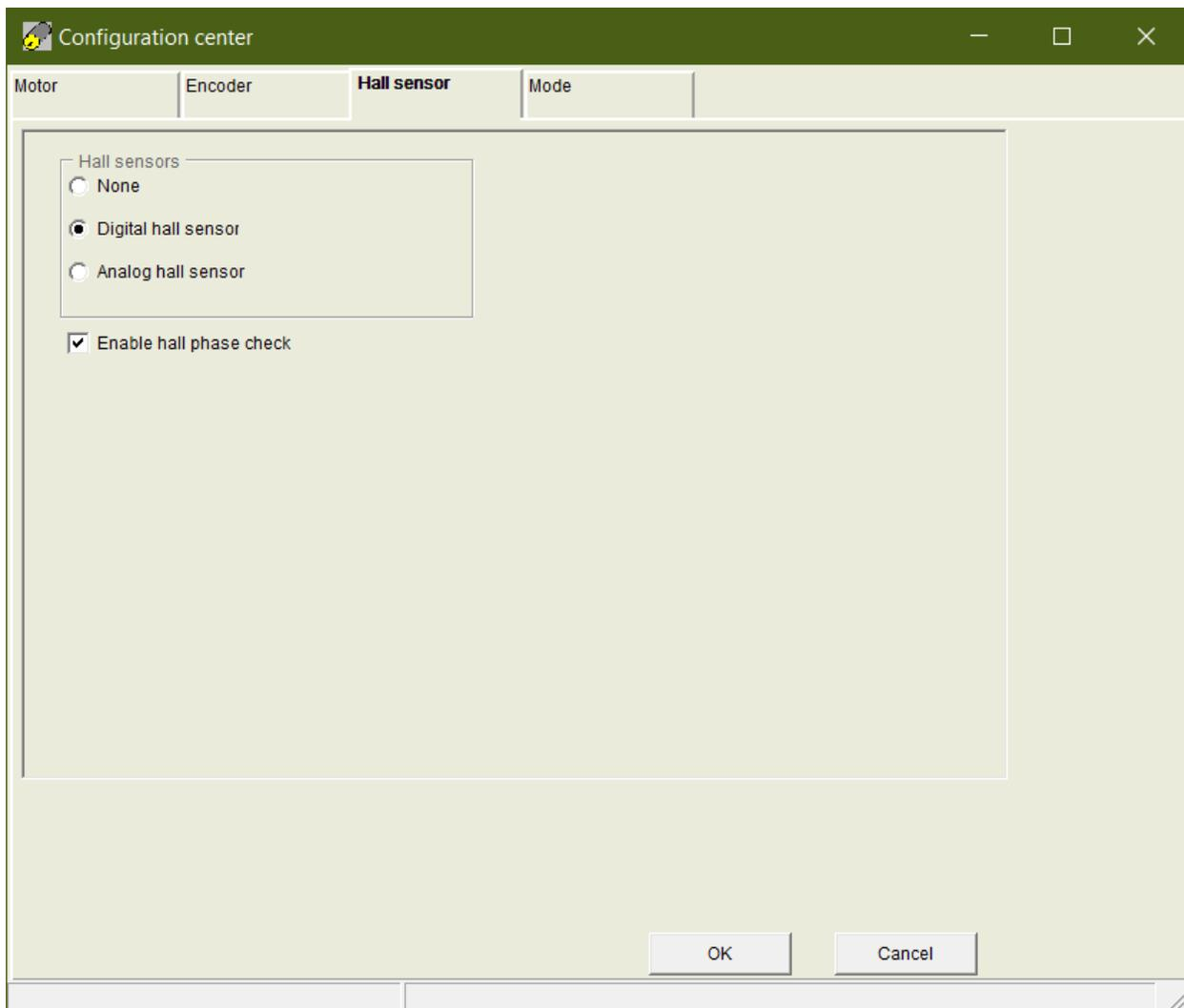
Figure 28: This figure illustrates the configuration of the linear motor's hall sensor.
