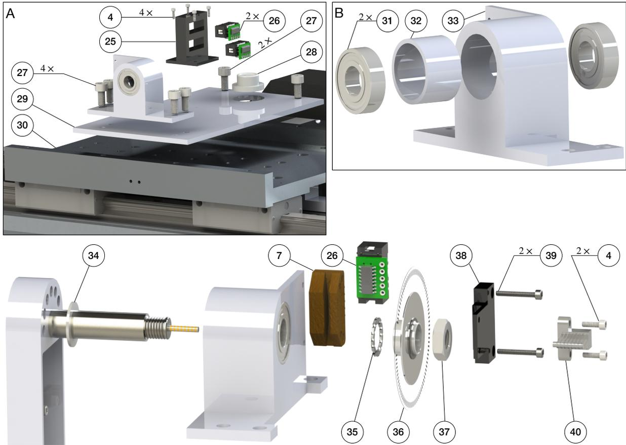
Figure 8: Assembly process of the pendulum cart, pendulum arm and bearing housing. (A) Installation of the bearing housing, cart plate and linear motor stage. (B) Assembly of the ceramic bearing and the bearing housing. (Bottom) Installation of the pendulum arm and bearing housing.
