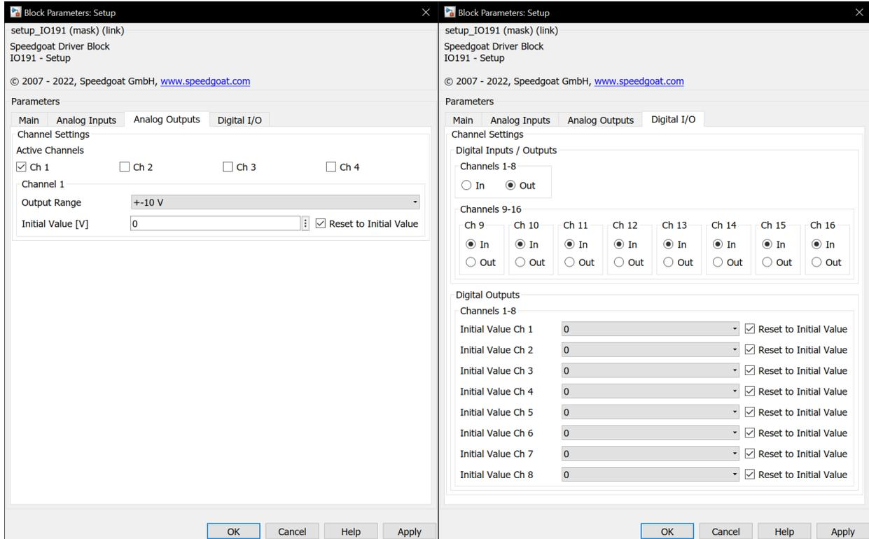
Figure 34: This figure illustrates the configuration of the IO-191 module's Simulink block. One of the analog signal outputs is selected to control the velocity of the pendulum cart in velocity mode. Meanwhile, eight ports of the digital I/O block are chosen as input ports, and the rest are set to output ports.
