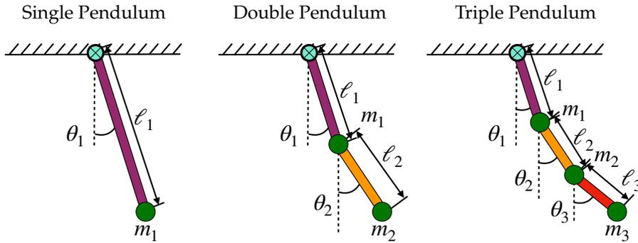
Figure 1: A schematic illustration of the single, double, and triple pendulum.
