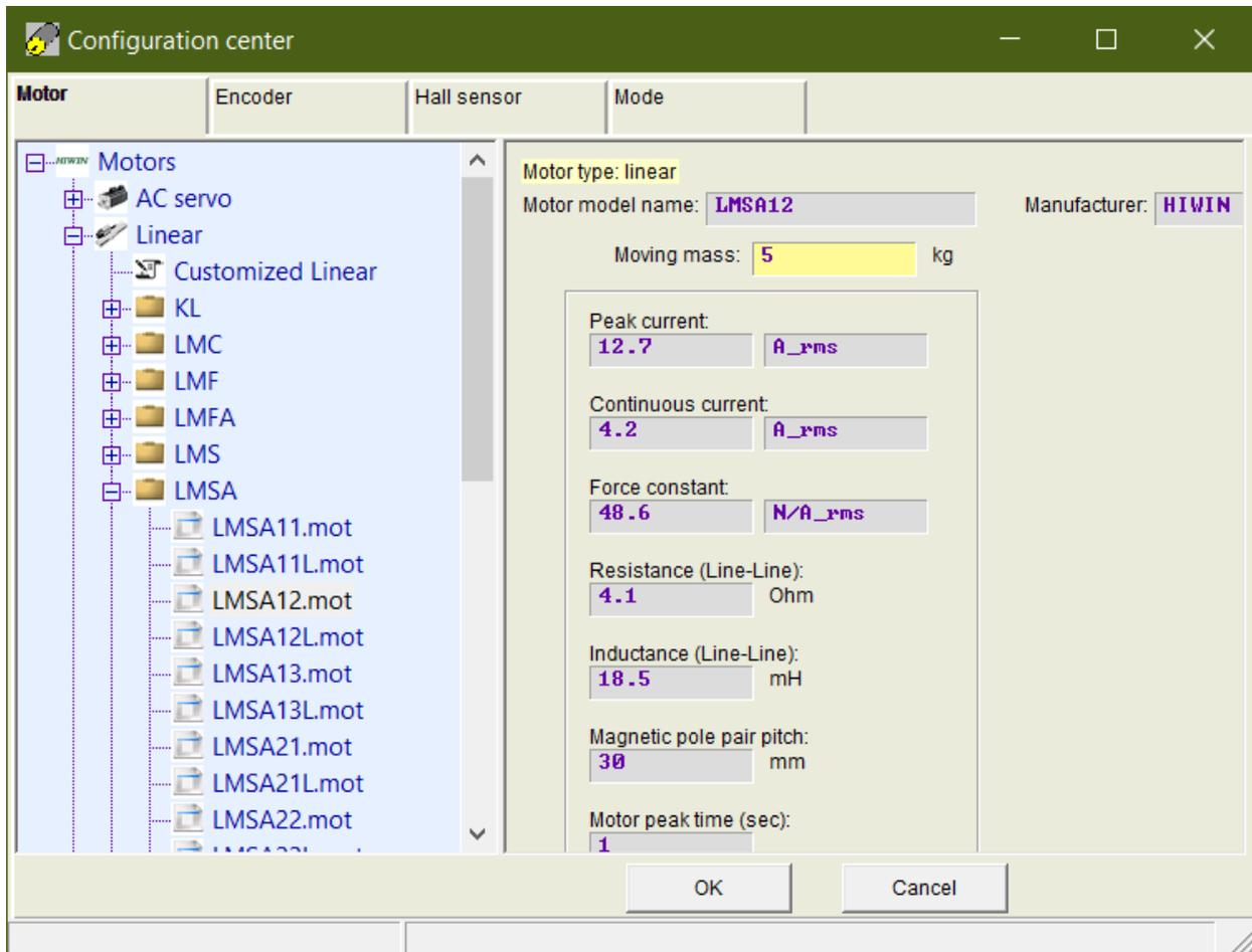
Figure 26: This figure illustrates the configuration of the motor parameters.
