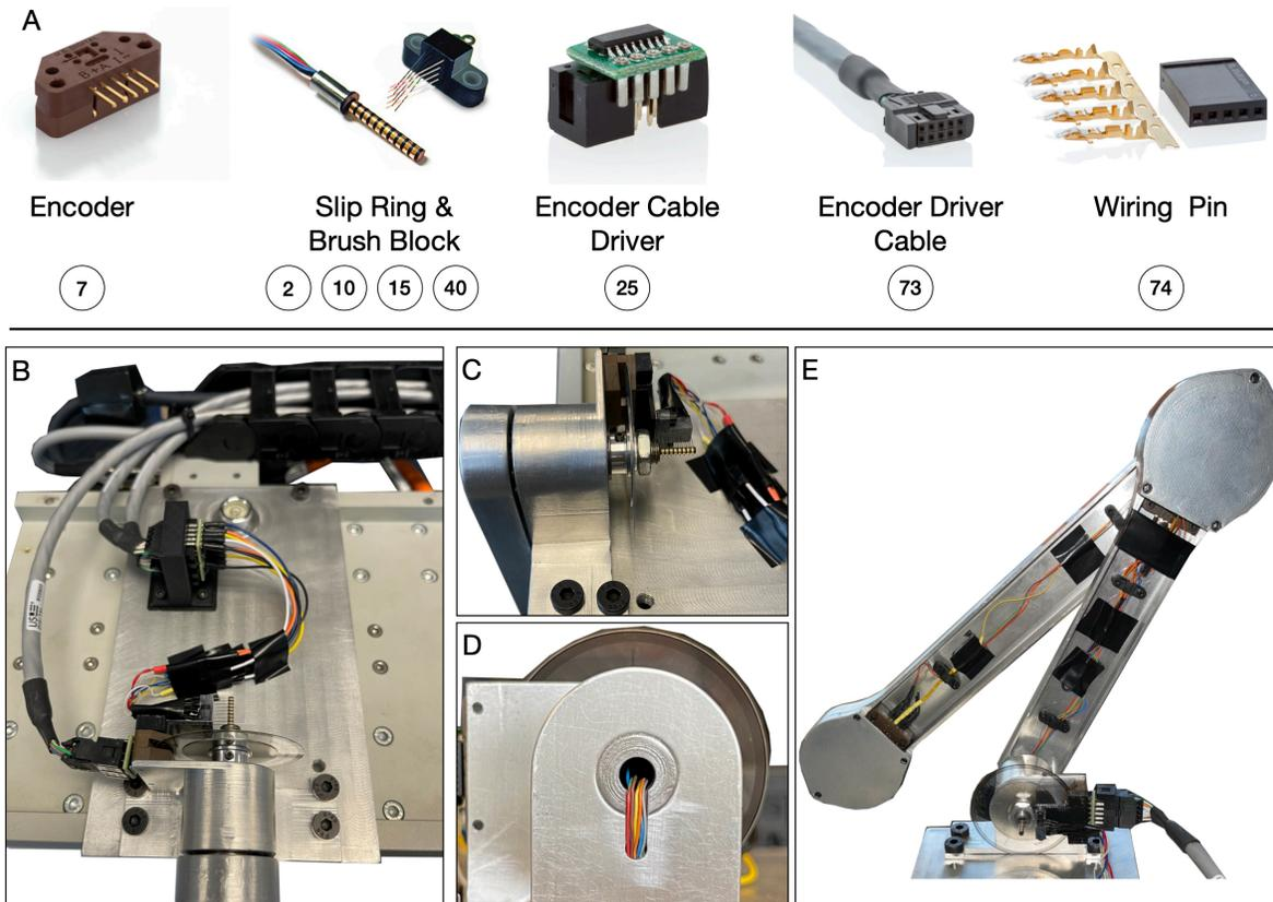
Figure 11: Electrical wiring and assembly of the pendulum arm. (A) Major electrical components of the pendulum arm. (B) connection method of differential driver and encoder reader. (C) to (E) wiring of the slip-ring.
