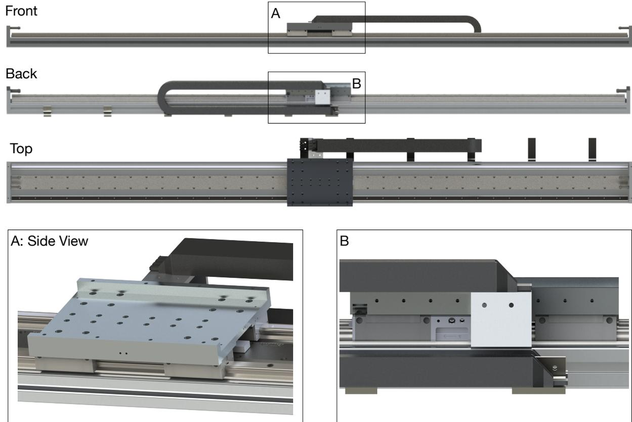
Figure 17: Overview of the linear motor that drives the pendulum cart, with the linear motor cable track and the stage with pre-drilled holes, which allow the installation of user designed parts. This linear motor stage is used to mount the aluminum plate that is used to install the bearing housing and the pendulum arm. (B) Limit switch plate installed on the back side of the linear motor stage.
