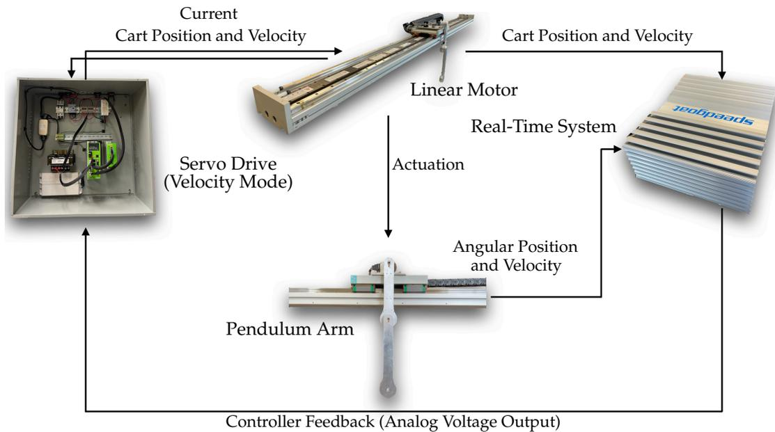
Figure 3: Closed loop control diagram of the proposed system. The linear motor and pendulum arm sends measurement data to the real-time system, which is used to calculate the corresponding control action needed to achieve the control object, such as stabilization, swing-up, stabilizing periodic orbit, etc. After the control command is received by the servo drive as an analog signal, the servo drive controls the linear motor to achieve the desired motion.
