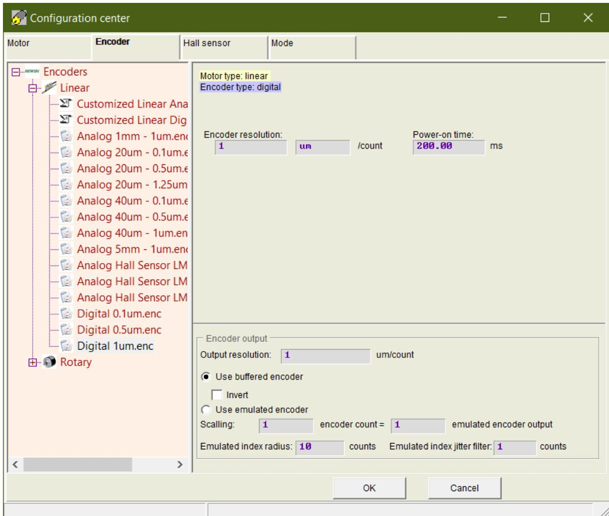
Figure 27: This figure illustrates the configuration of the linear motor’s encoder.
