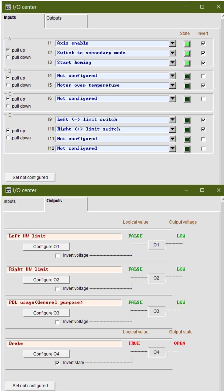
Figure 30: This figure illustrates the configuration of the HIWIN D1 drive's I/O functionalities.
