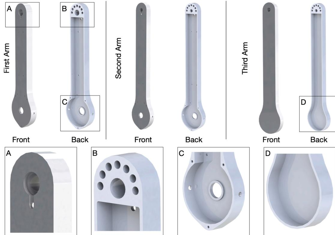
Figure 15: Design of the pendulum arm. (A) design features necessary to allow proper wiring of the slip-ring, and the hole where the pendulum shaft is installed. (B) back side of the pendulum where the shaft is installed, and a sequence of drilled holes that reduce the weight of pendulum arm. (C) place where the bearing and encoder are installed. (D) third pendulum arm without bearing hole.
