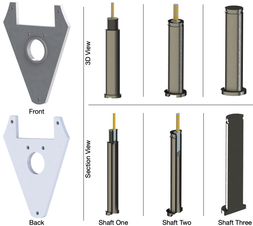
Figure 14: Design of the bearing plate and pendulum arm's shaft. The bearing can be installed on the bearing plate and together support the free rotational movement of the pendulum shaft and pendulum arm. The pendulum arm's shaft is designed hollow to accommodate the slip-ring wires. The groove on the bottom of the pendulum shaft is used to place guide the slip-ring wires into the pendulum arm.
