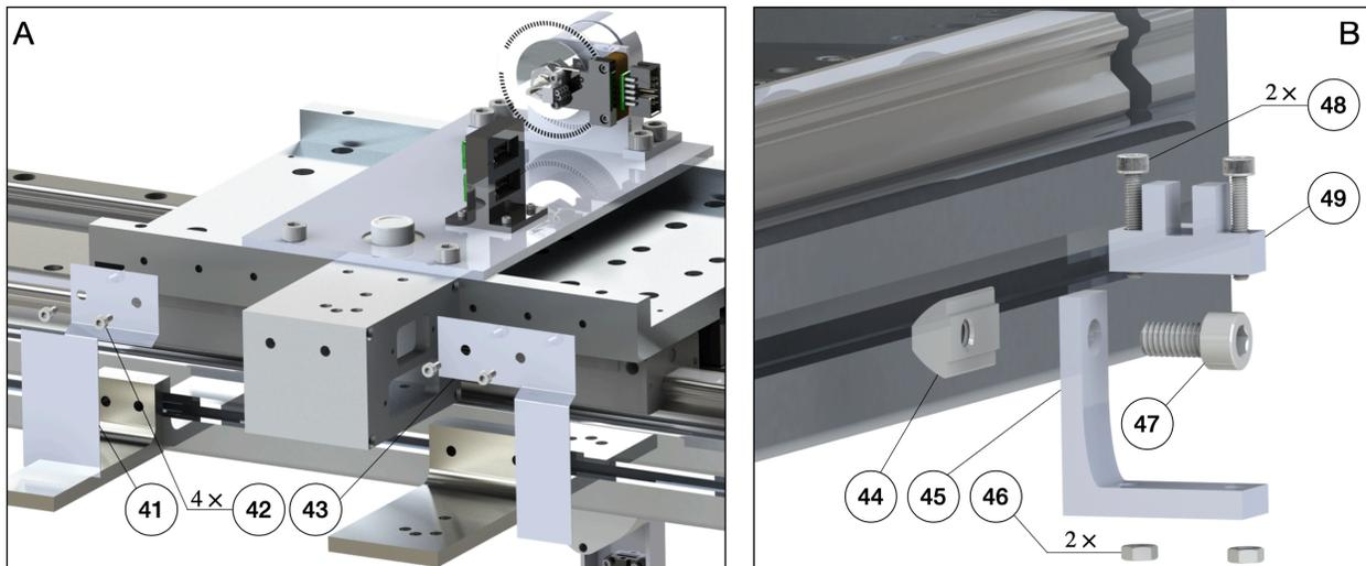
Figure 9: Assembly of the limit switch plate and limit switches.
