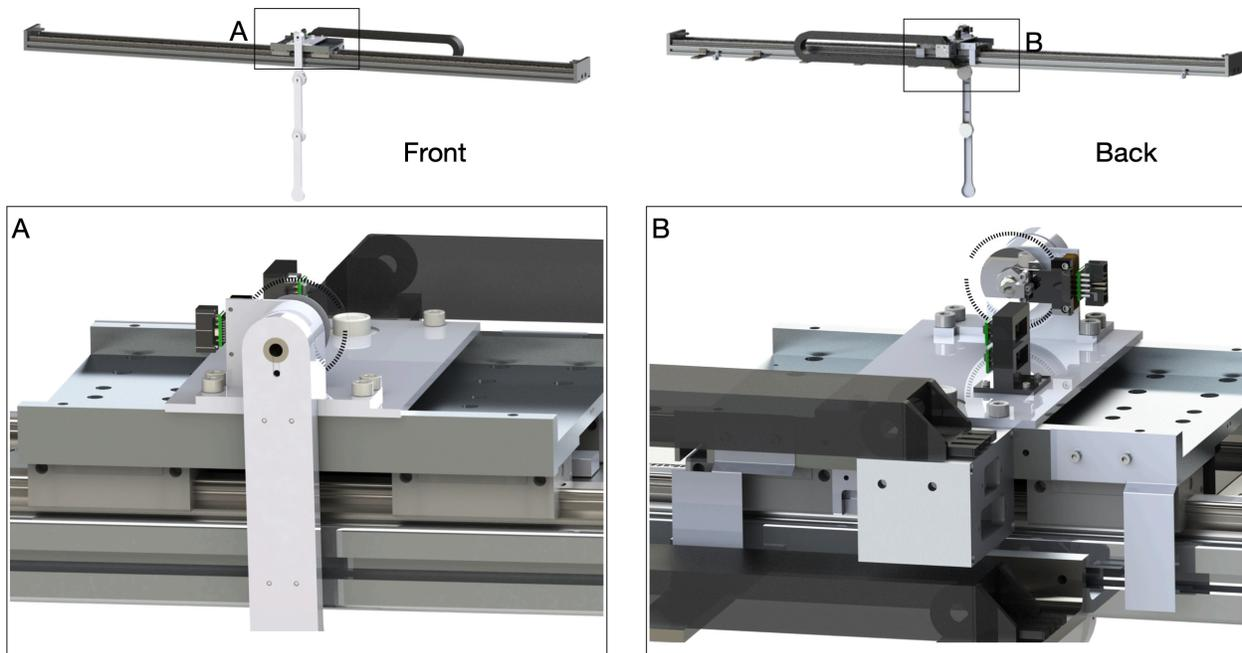
Figure 7: Overall assembly of the pendulum arm and pendulum cart. The main components of the pendulum cart are an aluminum plate and a bearing house.
