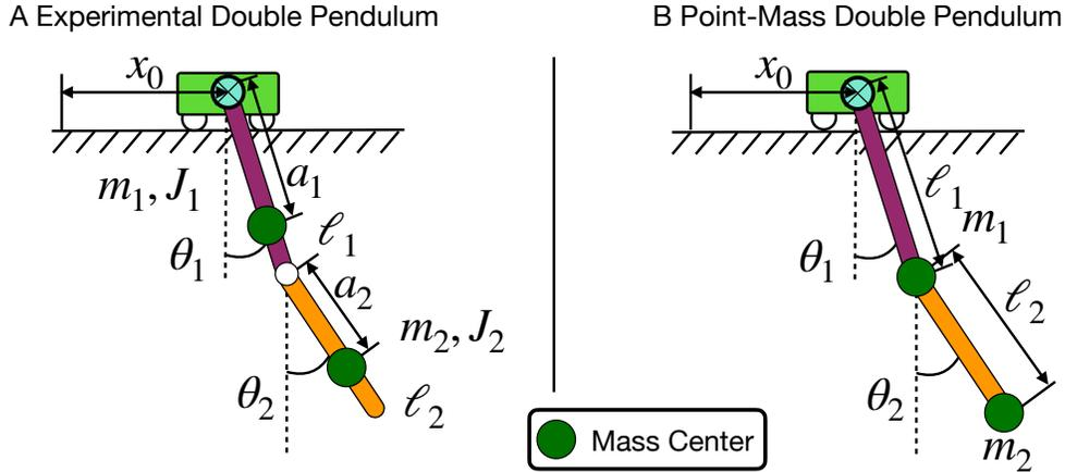
Figure 39: This figure illustrates the difference between the point-mass model of the double pendulum (left) and the more realistic experimental double pendulum (right) studied herein. The point-mass model ignores the mass of each arm of the pendulum, while the experimental model considers both the inertial ( $J_i$ ) and mass ( $m_i$ ) of the pendulum arms.
