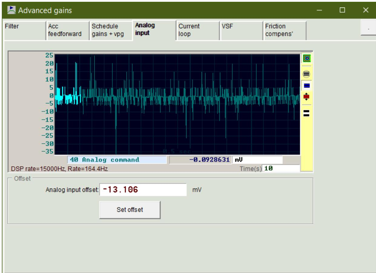
Figure 31: This figure illustrates the bias correction of the analog signal.
