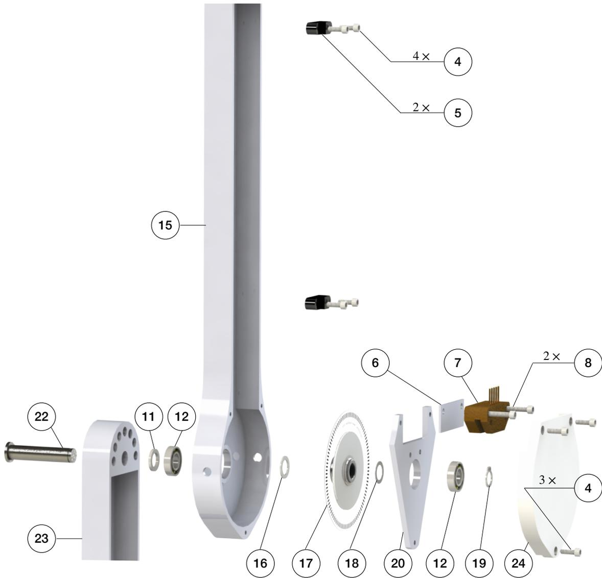
Figure 6: Components and assembly of the second and third pendulum arm.
