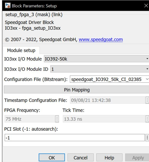
Figure 35: This figure illustrates the configuration of the IO-392 module’s Simulink block. The bitstream file provided by Speedgoat is needed to set up the IO-392 block to read encoder data properly.
