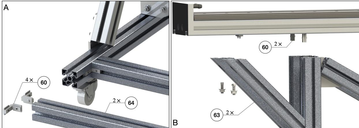
Figure 22: Assembly process of the system frame (A) and linear motor (B).
