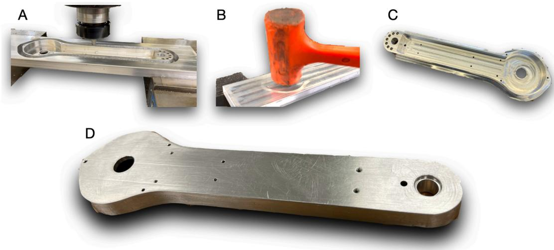
Figure 16: Overall steps needed to manufacture the pendulum arm: (A) the inside features of the pendulum arm is machined, and the outline of the pendulum arm is processed until only a thin layer of aluminium connects the pendulum arm and aluminium block. (B) and (C) the machined pendulum arm is knocked off using a rubber hammer. (D) the machined pendulum arm is polished to get rid of any burr on the edge of the pendulum arm.
