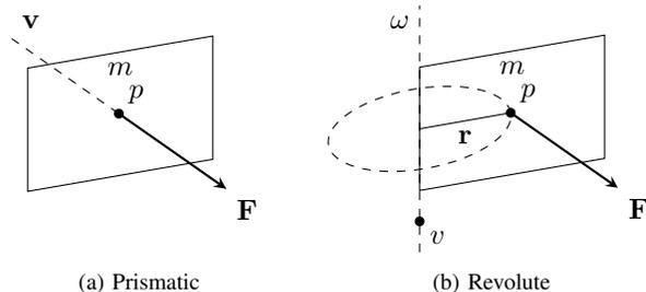
Fig. 2: Illustrations of prismatic and revolute joints.
