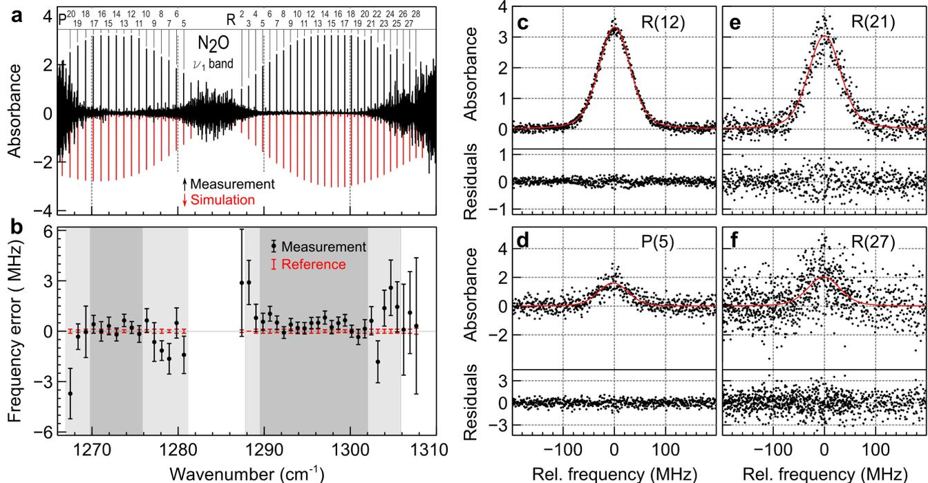
FIG. 3. **Spectra and retrieved line centers in a 54 ms acquisition** (a) Single shot spectra of the  $\nu_1$  fundamental band of nitrous oxide with 660 kHz spectral point spacing, acquired in 54-ms and comparison with simulation. (b) Retrieved line centers compared with literature reference with  $1\text{-}\sigma$  error bars. (c-f) Zoom of (e) on 4 different lines illustrating stronger/weaker absorbance and high/low SNR, and residuals of the Voigt fit shown in red.
