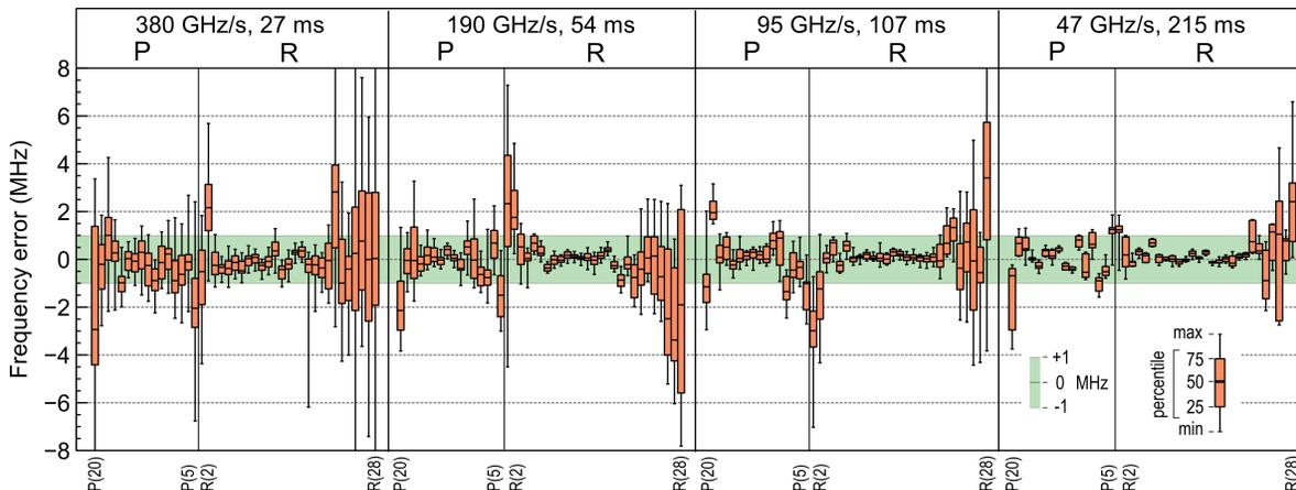
FIG. 4. **Frequency precision for varying scanning speed.** Frequency error and statistical spread of the retrieved line centers at 4 different scan speeds, decreasing from left to right by factors of 2. The precision increases with the scan time.
