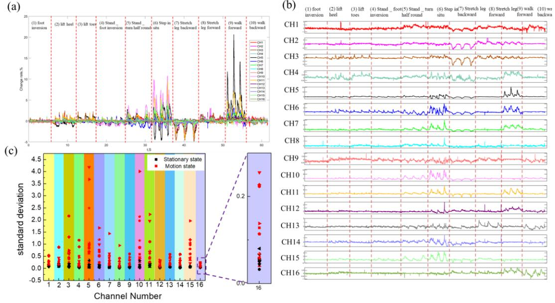
**Fig. 4. Response of the 16 channels of sensor elements to the ten lower limb motions.** (a) Real-time response of sensor array to multi-motions. (b) Response of each single channel to multi-motions. (c) Comparison of the standard deviation values of stationary state and motion state of the 10 different motions.
