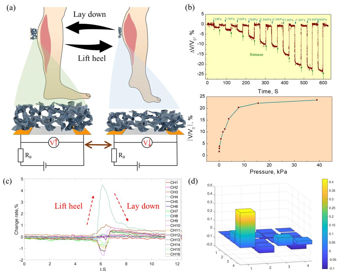
**Fig. 2. Response of the sensor array to pressures.** (a) Mechanism of sponge-based sensor detecting muscle deformation. (b) Response of individual sensory element to different applied pressure. (c) Response of all sixteen channels to the motions of lift heel and lay down with time. (d) Distribution of the mean value of rate of signal output change of the sensor array.
