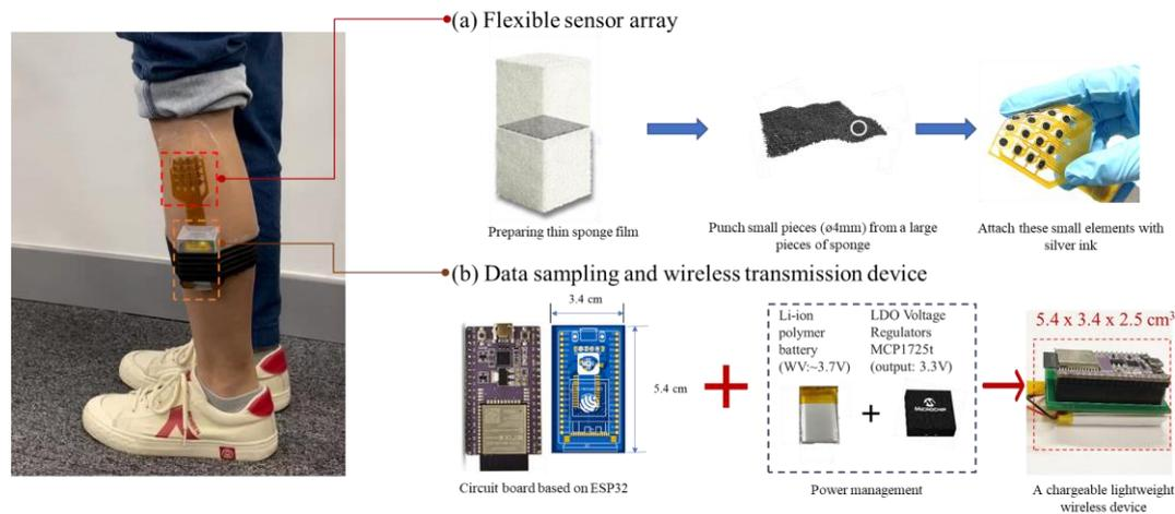
**Fig. 1. Structure of the whole portable motion detection device.** (a) Fabrication of the 16-channel sponge-based pressure sensor array. (b) Wireless circuit for data sampling and transmission.
