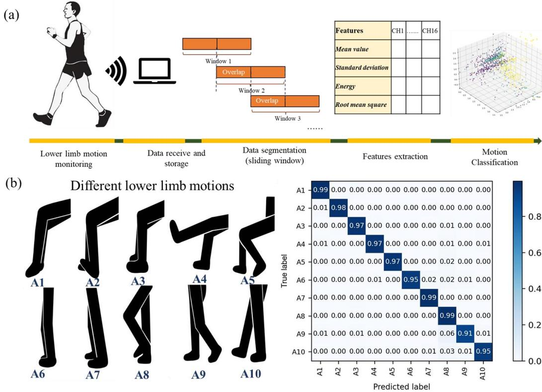
**Fig. 5. Recognition of ten kinds of different lower limb motions.** (a) Data process flow. (b) Classification results of ten different lower limb motions from ten human subjects (A1: lift heel, A2: lift toes, A3: foot inversion, A4: stretch leg forward A5: stretch leg backward, A6: standing with foot inversion, A7: turn round A8: step in situ, A9: walk forward, A10: walk backward).
