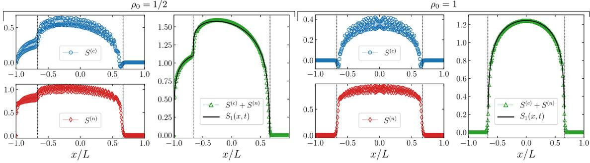
**Figure 10.** Configurational  $S^{(c)}$  and number  $S^{(n)}$  entanglement entropy as function of the cutting position  $x$  at time  $t/L = 0.67$ , for different initial states  $\rho_0 = 1, 1/2$  (see plots legend). The data are obtained for a system of 300 sites with exact lattice numerics, retaining only terms with  $|\Delta N| \leq 2$  in Eq. (80). The sum of the two contributions (symbols) is found in remarkable agreement with the hydrodynamic prediction in Eq. (61) (solid line).
