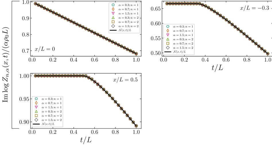
**Figure 6.** Imaginary part of the charged moments as function of time for different cutting position  $x$  (panels) and values of  $\alpha$ ,  $n$  (see plots legend). The hydrodynamic prediction in Eq. (67) is found in agreement with exact numerical data obtained for a system of size 300.
