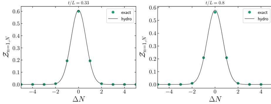
**Figure 7.** Symmetry-resolved partition function in Eq. (68) at half system ( $x = 0$ ) as function of  $\Delta N$ , at  $n = 1$  and at different times  $t/L = 0.33, 0.8$  (see plots legend). In each plot, the symbols show the numerical data obtained for a lattice of 300 sites while the solid line is the analytical prediction in (71).
