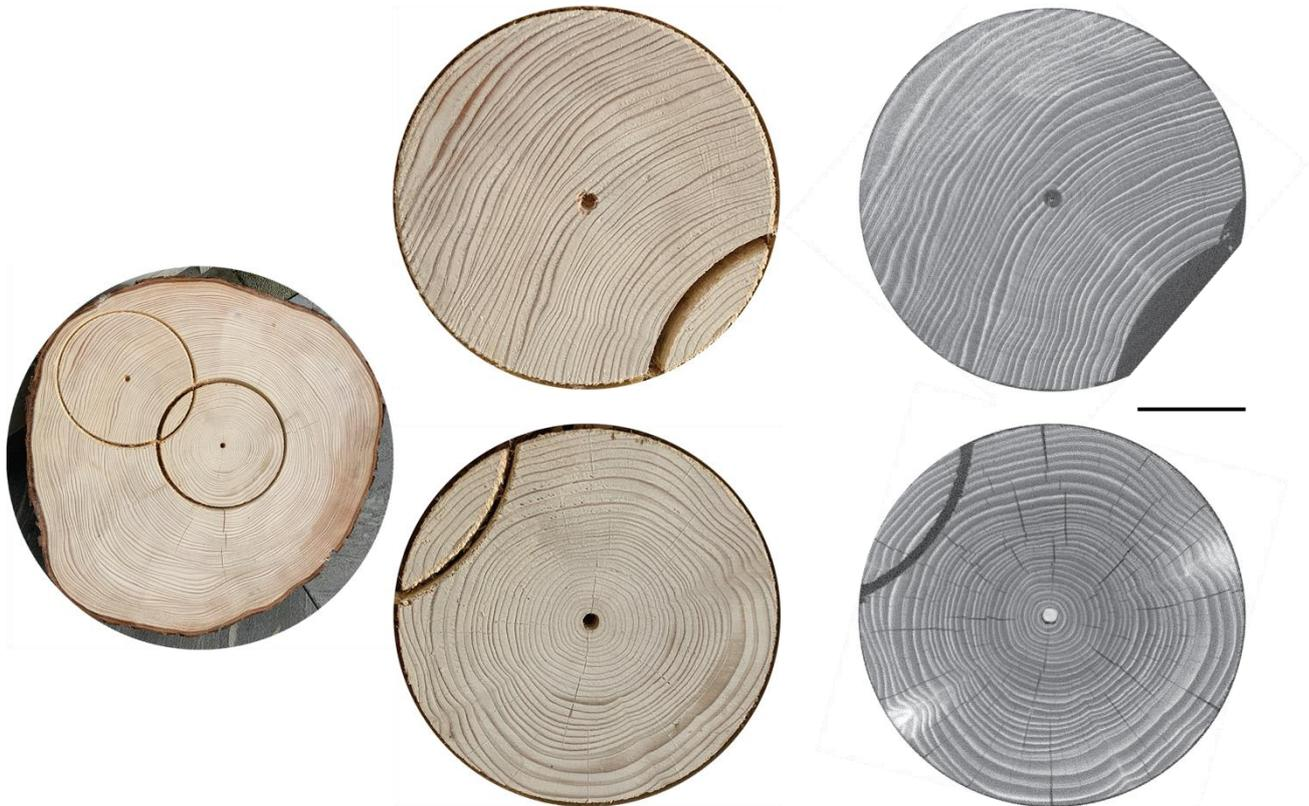
Figure 2. For the tomographic imaging using X rays, two cylinders with a diameter of 180 mm each were prepared, see photographs. The related tomography slices near the surface are represented on the right. The length bar corresponds to 50 mm.
