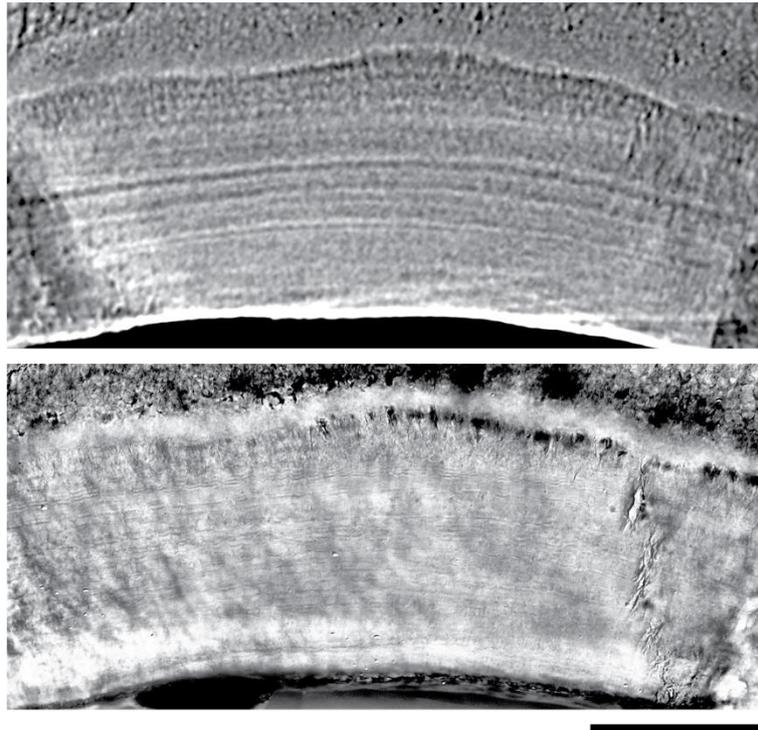
Figure 7. Comparison of incremental layer appearance for same region using hard X-ray tomography (top image) and optical imaging (bottom image). The length bar corresponds to 100  $\mu\text{m}$ .
