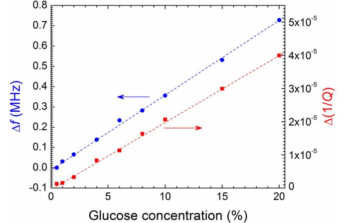
Fig. 4. Resonance frequency shift (circles) and changes in inverse  $Q$ -factors (squares) dependencies on concentration of glucose in aqueous solution.
