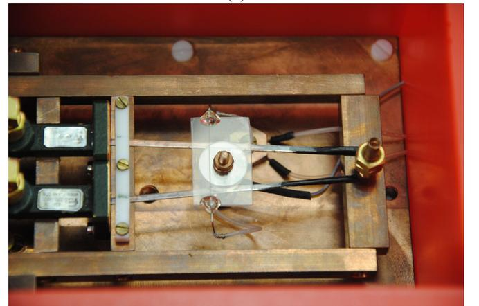
Fig. 1. Measurement cell consisting of WGM resonator with a plastic layer and a microfluidic channel, a pair of dielectric waveguides with coaxial-to-waveguide transitions in a thermally stabilized box: (a) – schematic, (b) – photo.
