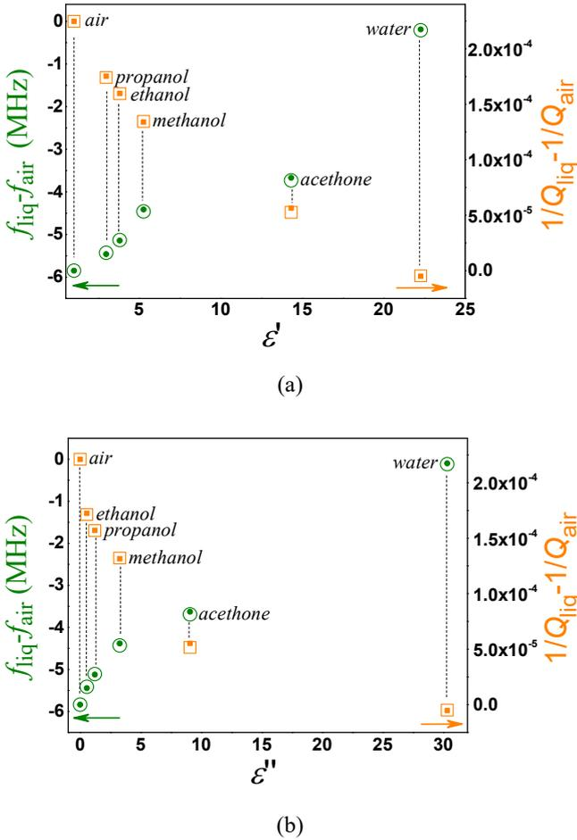
Fig. 3. Resonance frequency shift (circles) and changes in inverse  $Q$ -factors (squares) as a function of: (a) real and (b) imaginary parts of permittivity. The solid points present experimental data, open points calculated ones and dashed lines link data corresponding to the certain liquid.
