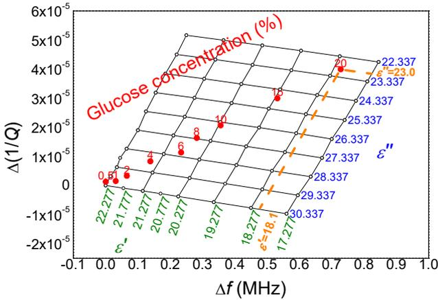
Fig. 5. Nomogram chart. Calculated net for the resonant frequency shift and changes in the inverse quality factor for a microfluidic channel filled with substances with varying real and imaginary parts of the permittivity (see text for details). Red points show the experimentally obtained data for resonant frequency shift and changes in inverse  $Q$ -factor as functions of glucose concentration in water solution.
