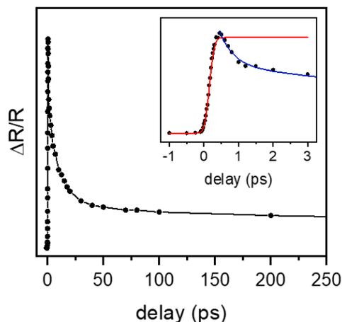
**Figure S2. Normal incident pump-probe experiment using a 515 nm pump and 730 nm probe.** The inset shows the early pump-probe time delay signal. The estimated instrument response function from the fit is 129 fs.
