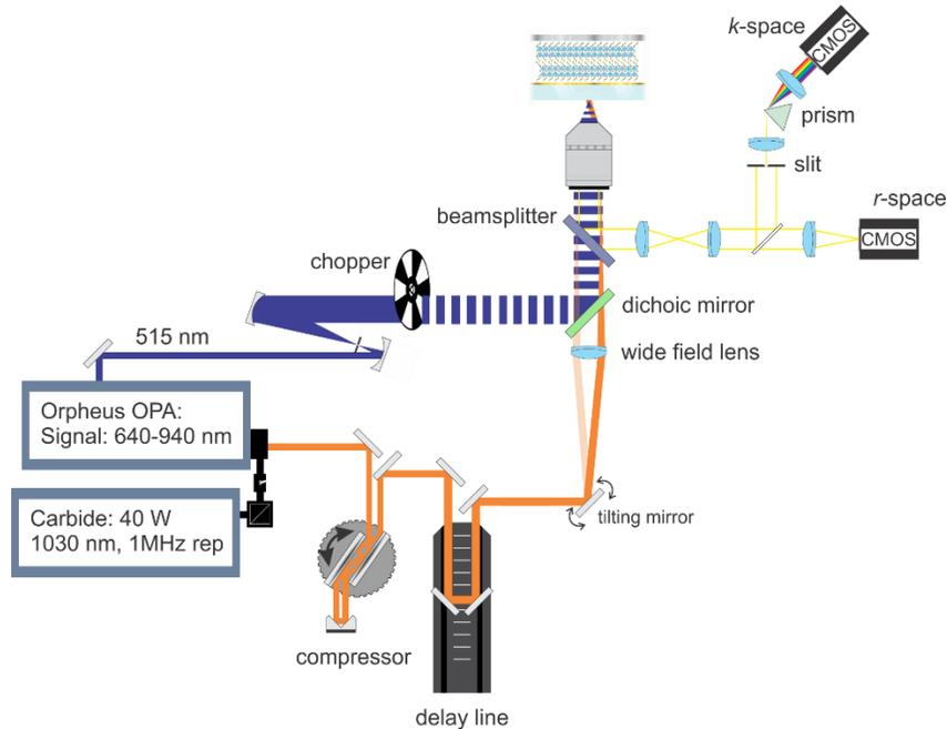
**Figure S1. MUPI schematic.** Optical schematic for momentum-resolved ultrafast polariton imaging.
